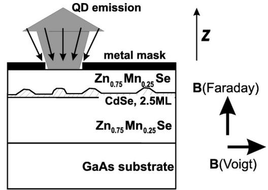
FIG. 1. A sketch of the sample with a metal aperture. Directions of the magnetic field in “Faraday” and “Voigt” geometries are shown by arrows.
