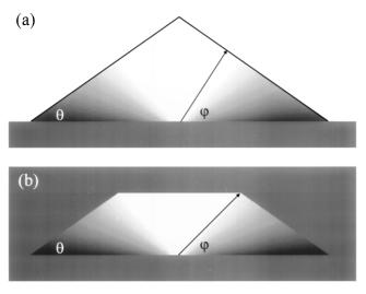
FIG. 3. Theoretical concentration profiles [Eq. (2)] displayed in gray scale. (a) Triangular island. (b) Buried quantum dot. We assume that capping simply dissolves the island apex and surrounds the dot with GaAs.
