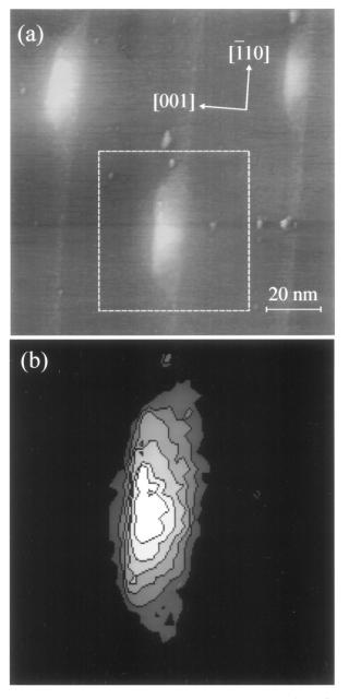
FIG. 1. (a) A 120 nm  $\times$  120 nm STM image obtained from (110) cleavage surface. The growth surface is toward the left. Within a QD the bright triangular shape with the base at the top of the dot indicates the nonuniform distribution of In atoms. The gray scale displayed is 5.5 Å. (b) Contour plot of the middle QD [frame marked in (a)]; contour intervals are 0.5 Å.
