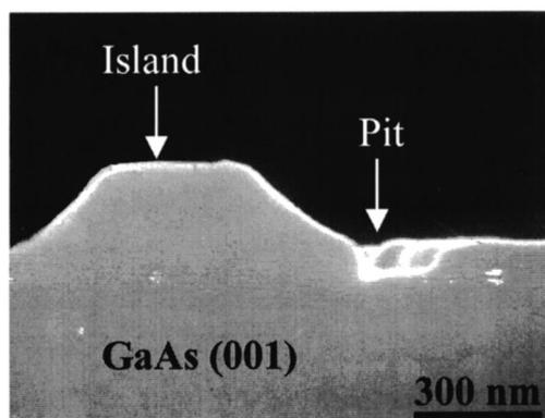
FIG. 5. A cross-sectional SEM image of an island–pit combination in the 40 nm thick layer.
