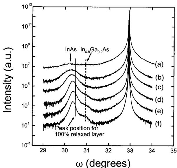
FIG. 4. X-ray double-crystal 004 rocking curves of the six samples. Curves (a)–(f) correspond to layers with thicknesses of 4, 10, 20, 40, 60, and 80 nm. The solid line indicates the position where the InAs peak should be if the layer is completely strain relaxed. The dashed line indicates the position of the shoulder peak.
