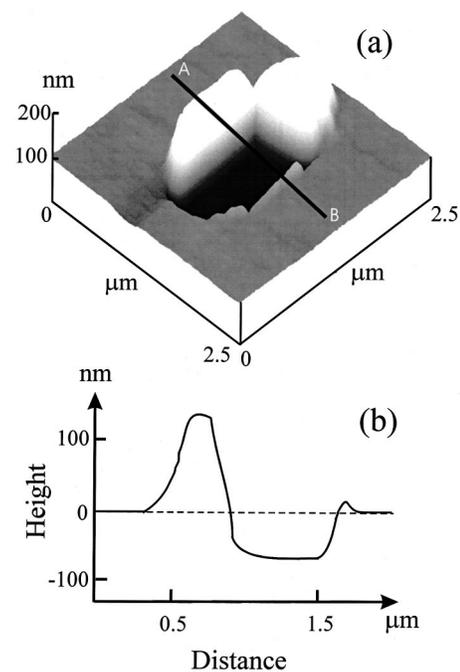
FIG. 3. (a) A small area AFM image taking from the 40 nm thick layer, and (b) the corresponding AFM cross-sectional analysis.
