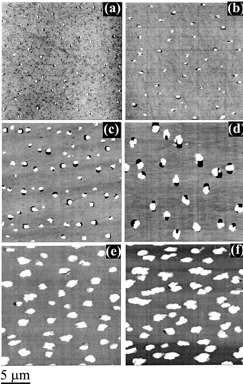
FIG. 1. AFM images of six InAs layers grown on GaAs (001) substrates. The layer thicknesses are (a) 4 nm, (b) 10 nm, (c) 20 nm, (d) 40 nm, (e) 60 nm, and (f) 80 nm, respectively.
