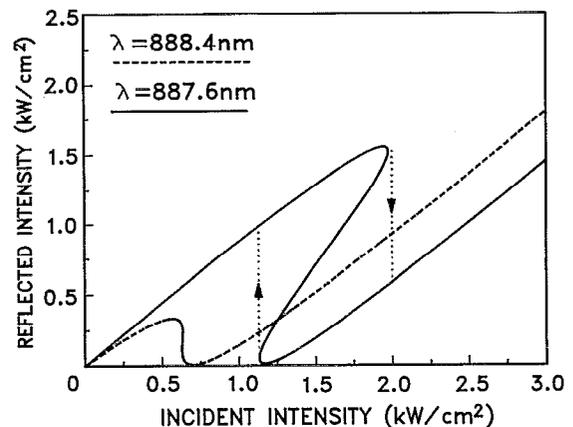
FIG. 2. Reflected-versus-incident intensity characteristics of the structure for two different wavelength detunings.
