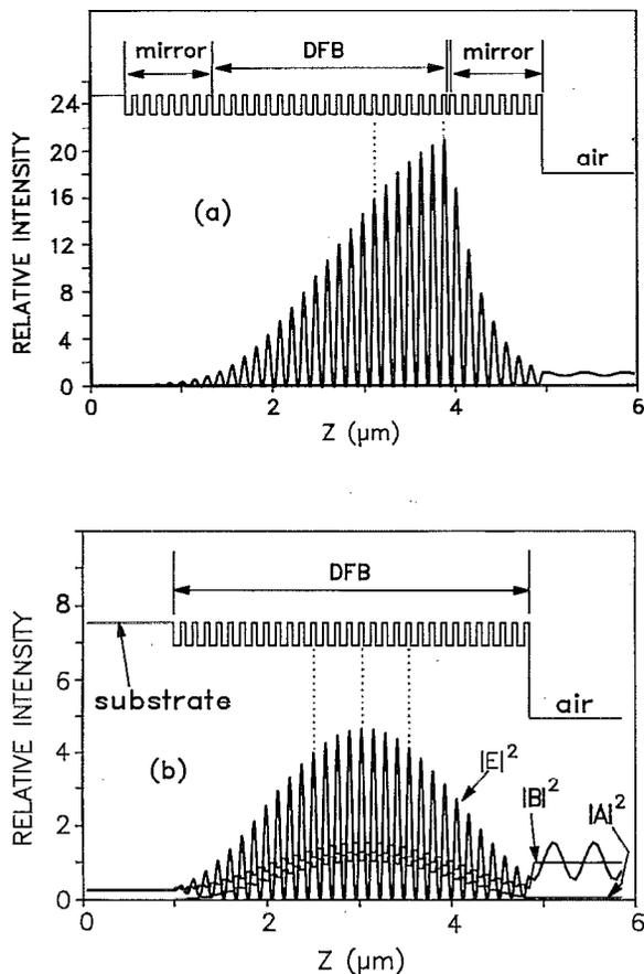
FIG. 3. Intensity distribution in the combined DFB/FP structure (a) and in the DFB structure considered in Ref. 4(b) at resonant wavelengths. The amplitude of the incident beam is normalized to 1. The top curve shows the refractive index profile of the structure. The squared module of the forward and backward wave amplitudes are also shown in (b).
