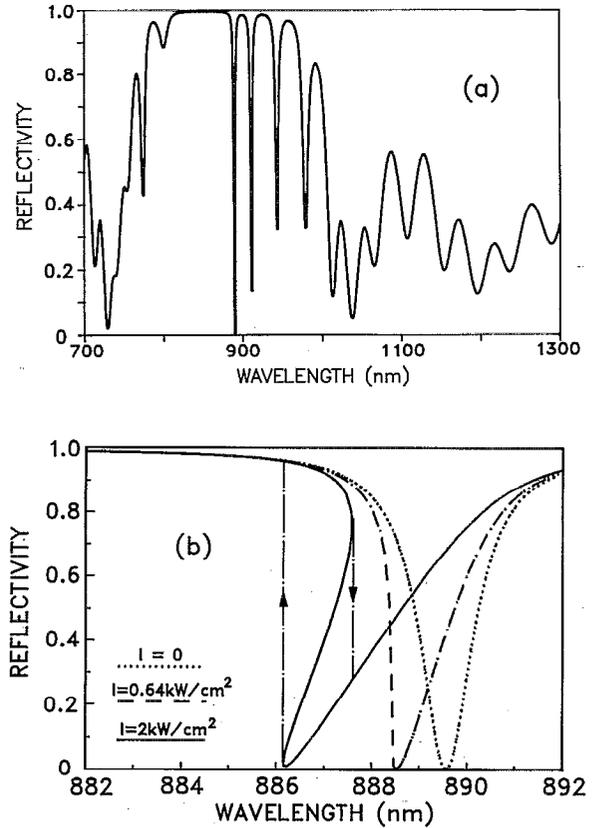
FIG. 1. Linear (a) and nonlinear (b) reflectivity spectra of the combined DFB/FP structure.
