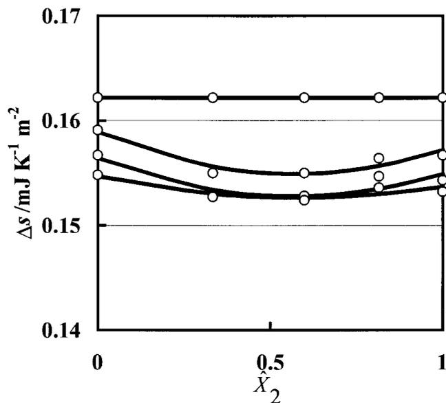
FIG. 7. Entropy of surface formation-versus-composition of the mixtures at constant total concentrations. The total concentration of the curves are 0.0, 0.5, 1.0, 1.5 mol kg<sup>-1</sup> from top to bottom.
