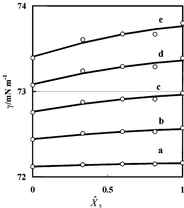
FIG. 3. Surface tension-versus-composition relations of the mixtures at constant concentrations: (a)  $\hat{m} = 0.2 \text{ mol kg}^{-1}$ ; (b) 0.6; (c) 1.0; (d) 1.4; (e) 1.8.
