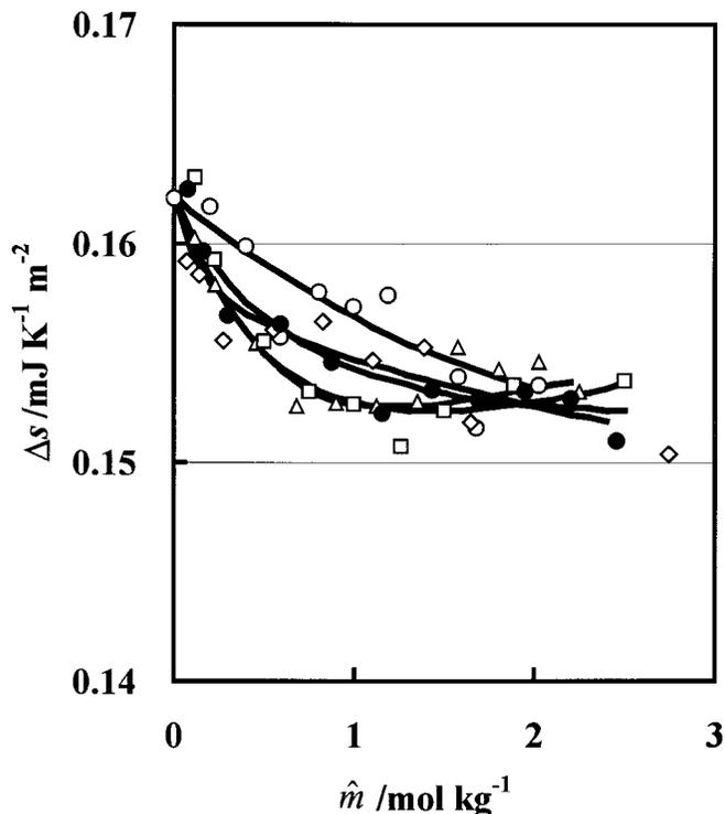
FIG. 6. Entropy of surface formation-versus-total concentration curves of the mixtures at constant composition: (○)  $\hat{X}_2 = 0.00$ ; (△) 0.33; (□) 0.60; (◇) 0.82; (●) 1.00.
