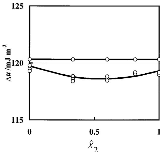
FIG. 8. Entropy of surface formation-versus-composition of the mixtures at constant total concentrations. The total concentration of the curves are 0.0, 0.5, 1.0, 1.5 mol kg<sup>-1</sup> from top to bottom.
