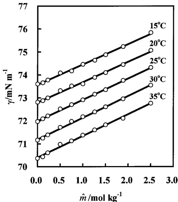
FIG. 1. Surface tension-versus-total molality relations of the mixture of  $\hat{X}_2 = 0.60$  at constant temperatures.
