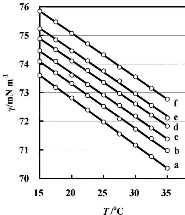
FIG. 2. Surface tension-versus-temperature relations of the mixture of  $\hat{X}_2 = 0.60$  at fixed concentrations: (a)  $\hat{m} = 0.00$  mol  $\text{kg}^{-1}$ ; (b) 0.50; (c) 1.00; (d) 1.50; (e) 1.89; (f) 2.50.
