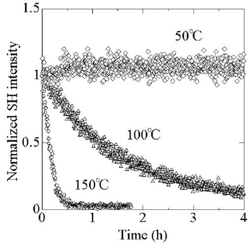
**Figure 3.** Decay of second-harmonic intensity for  $15\text{Nb}_2\text{O}_5\cdot 85\text{TeO}_2$  glass doped with  $\text{Na}^+$ . The glass was thermally poled at  $260^\circ\text{C}$ . The measurements of decay were carried out at  $50^\circ\text{C}$  ( $\square$ ),  $100^\circ\text{C}$  ( $\triangle$ ), and  $150^\circ\text{C}$  ( $\circ$ ).
