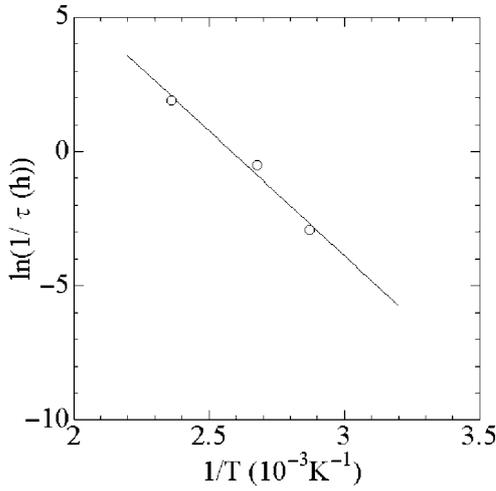
**Figure 5.** Temperature dependence of relaxation time for Na<sup>+</sup>-doped 15Nb<sub>2</sub>O<sub>5</sub>·85TeO<sub>2</sub> glass poled at 260°C. The straight line was drawn by the least-squares method.
