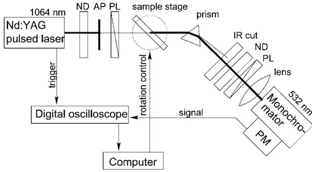
**Figure 2.** A schematic illustration of equipment for measurements of second-harmonic generation in thermally poled  $15\text{Nb}_2\text{O}_5\cdot 85\text{TeO}_2$  glass. The Maker fringe method was used for the SHG measurements. The abbreviations, i.e. ND, AP, and PL denote neutral density filter, aperture, and polarizer, respectively.
