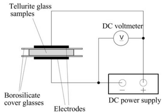
**Figure 1.** A schematic illustration of apparatus for thermal poling of 15Nb<sub>2</sub>O<sub>5</sub>-85TeO<sub>2</sub> glass.
