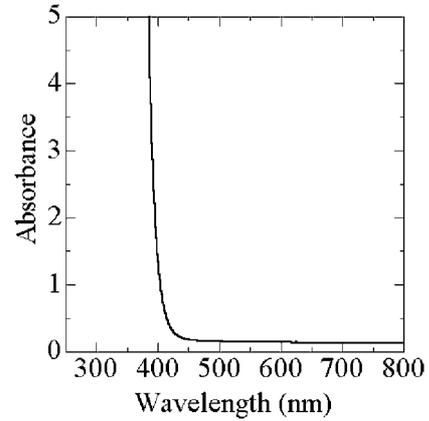
**Figure 6.** Room temperature optical absorption spectrum of 15Nb<sub>2</sub>O<sub>5</sub>·85TeO<sub>2</sub> glass before optical poling.
