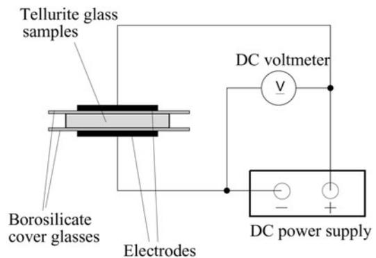
**Figure 1.** A schematic illustration of apparatus for thermal poling of 15Nb<sub>2</sub>O<sub>5</sub>-85TeO<sub>2</sub> glass.
