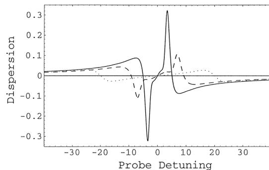
Fig. 4. The steady state results for dispersion  $\text{Re}(\sigma_{31})/E$  as a function of the probe detuning  $\Delta_3$  for the same parameters as in Fig. 2 but with no incoherent pumping ( $R = 0$ ). Dotted curve shows results with  $p = 0$ , dashed curve with  $p = 0.95$  and finally solid curve with  $p = 0.99$ .
