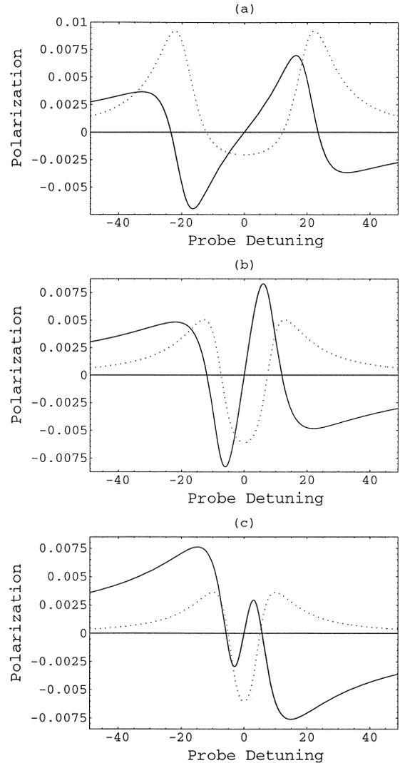
Fig. 2. The steady state results for absorption  $\text{Im}(\sigma_{31})/E$  (dotted line) and dispersion  $\text{Re}(\sigma_{31})/E$  (solid line) as a function of the probe detuning  $\Delta_3$  for parameters  $\Delta_2 = 0, E_0 = \gamma_3, \Omega_0 = 20\gamma_3, \gamma_2 = 6\gamma_3, R = 2\gamma_3$ . (a)  $p = 0$ , (b)  $p = 0.95$  and (c)  $p = 0.99$ .  $\Delta_3$  is measured in units of  $\gamma_3$ .
