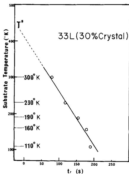
Fig. 6. Length of second resident time vs substrate temperature for 33L glass containing 30% crystallization.
