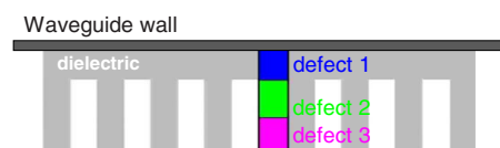
FIG. 1. (Color online) Schematic of the 1D periodic structures (side view) with corrugated dielectric insert (the air, dielectric, and waveguide walls are shown by the white, gray, and black colors) with localized "zero" length defects of the period. Defect 1 has a radius equal to the maximum radius of the corrugation; defect 2 has an intermediate radius; and defect 3 has a radius equal to the minimum corrugation radius.
