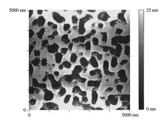
FIG. 10. AFM image of a 5  $\mu$ m $\times$ 5  $\mu$ m portion of the luminescing region of a SIMOX sample following removal of the upper oxide with buffered oxide etch. The large pits in the image arise from regions in which the entire thickness of the Si layer had been oxidized, allowing the etchant to attack the buried oxide.
