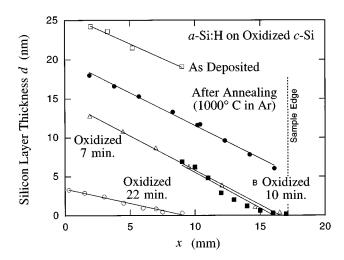
FIG. 8. Silicon layer thickness profiles of a-Si:H sample D taken after a-Si:H deposition ( $\square$ ), after annealing/crystallization ( $\blacksquare$ ), after 7 min in O<sub>2</sub> at 1000 °C ( $\triangle$ ), after a total of 10 min of oxidation ( $\blacksquare$ ), and after a total of 22 min of oxidation ( $\bigcirc$ ).
