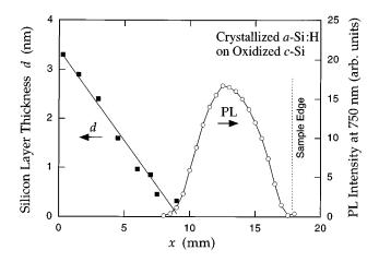
FIG. 6. Plot of the mean layer thickness d and the peak PL intensity at  $\lambda = 750$  nm as functions of position x of a-Si:H sample D. Virtually no PL is observed in the region of non-negligible thickness, as determined from the reflection spectra.
