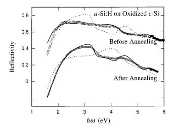
FIG. 2. Reflection spectra of crystallized a-Si:H sample D taken after annealing in Ar to  $1000\,^{\circ}$ C and oxidation in 1 atm  $O_2$  at  $1000\,^{\circ}$ C for 7 min. Symbols are data; smooth curves are fits, which assume that the Si layer is fully crystalline.
