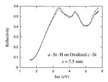
FIG. 7. Reflection spectrum at x=7.5 mm on a-Si:H sample D. The solid curve is a fit using the index of refraction of bulk c-Si, giving an estimated thickness of 0.5 nm. The dashed curve fit is a fit using the dielectric function of 0.6-nm-thick c-Si taken from Ref. 36, which gives 1.2 nm for the Si layer thickness.
