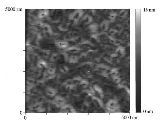
FIG. 9. AFM image of a  $5 \,\mu \text{m} \times 5 \,\mu \text{m}$  region of a SIMOX sample made when the average Si layer thickness measured by reflectivity was  $\sim 10 \, \text{nm}$ . The rms roughness of this image is  $\sigma = 2.25 \, \text{nm}$ .
