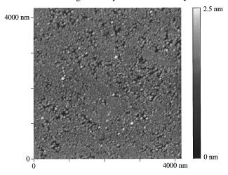
FIG. 12. AFM image of a 5  $\mu$ m $\times$  5 $\mu$ m area in the luminescent region of the sample shown in the previous figure.
