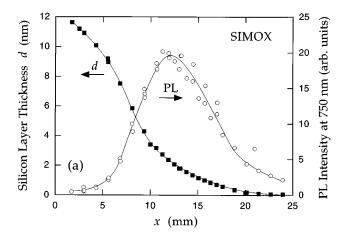
FIG. 5. Plot of the mean layer thickness d and the peak PL intensity at  $\lambda = 750$  nm as functions of position x on the triple-implant SIMOX sample of Fig. 2, showing a peak luminescence intensity for a thickness of  $\sim 2$  nm. (b) Crystallized a-Si:H layer on oxidized c-Si. Virtually no PL is observed in the region of nonnegligible thickness as seen in reflection spectra.
