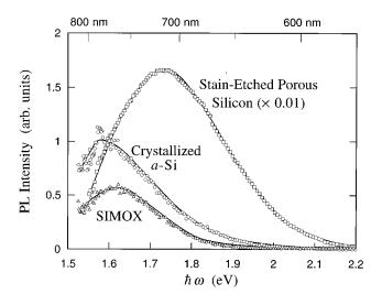
FIG. 3. Photoluminescence (PL) spectra of thin Si layers made from a SIMOX substrate ( $\blacktriangle$ ), crystallized a-Si:H deposited on an oxidized c-Si substrate ( $\bigcirc$ ), and of a stain-etched porous Si layer ( $\blacksquare$ ). The excitation source was an Ar<sup>+</sup> laser (488 nm, 2.54 eV) and the spectra were corrected for instrumental response. Smooth curves are guides to the eye.
