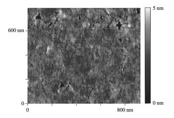
FIG. 11. AFM image of a 1  $\mu$ m $\times$  1  $\mu$ m portion crystallized a-Si:H layer that was thinned by oxidation at 1000 °C. The mean layer thickness determined from reflection spectra was  $\sim$ 1 nm in the imaged region.
