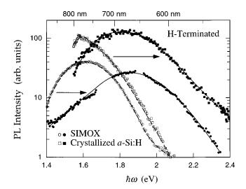
FIG. 14. PL spectra taken following the removal of the upper oxide layer with pH-buffered HF (filled symbols) are shifted  $\sim$ 0.3 eV to higher energy compared to those taken with the oxide layer intact (open symbols). The same behavior was observed with SI-MOX samples (squares) and crystallized a-Si:H layers (circles).
