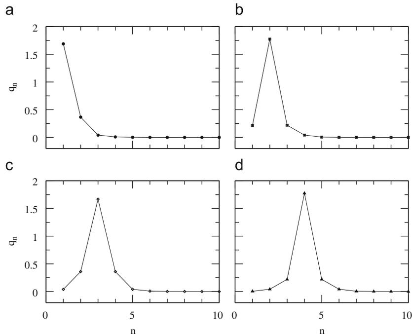
Fig. 2. Typical Hamiltonian single-site surface breather profiles at maximum amplitude in a magnetoinductive binary array for  $\delta = 0.9$ ,  $\lambda = 0.1$ ,  $\omega = 0.77$ ,  $\chi = +\frac{1}{6}$ ,  $N = 40$ .
