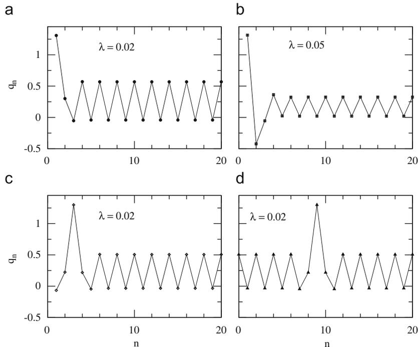
**Fig. 3.** Dissipative low-amplitude surface breather profiles at maximum amplitude for  $\delta = 0.8$ ,  $\Omega = 0.92$ ,  $\chi = +\frac{1}{8}$ ,  $\gamma = 0.01$ ,  $\epsilon_0 = 0.04$ ,  $N = 40$ , and  $\lambda$  as shown in the figure. The central breather site is located on an odd-numbered SRR oscillator.
