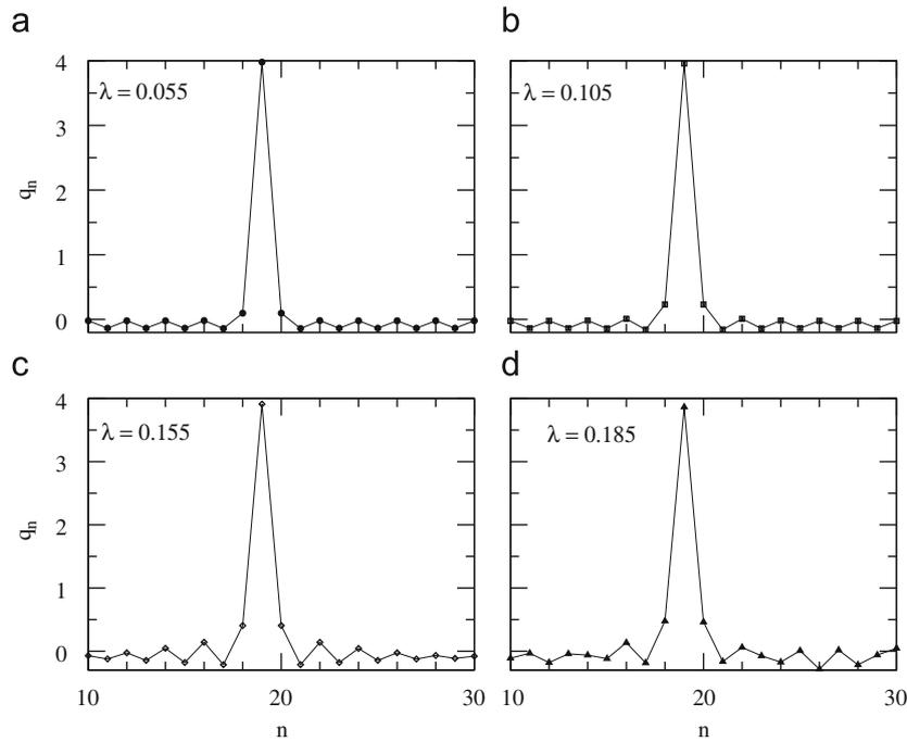
**Fig. 4.** Dissipative, high-amplitude bulk breather profiles at maximum amplitude for  $\delta = 2$ ,  $\Omega = 0.5$ ,  $\chi = +\frac{1}{6}$ ,  $\gamma = 0.01$ ,  $\epsilon_0 = 0.04$ ,  $N = 40$  and different values of the coupling parameter  $\lambda$  as shown in the figure. The central breather site is located on an odd-numbered SRR oscillator ( $n = 19$ ) in the middle of the array.
