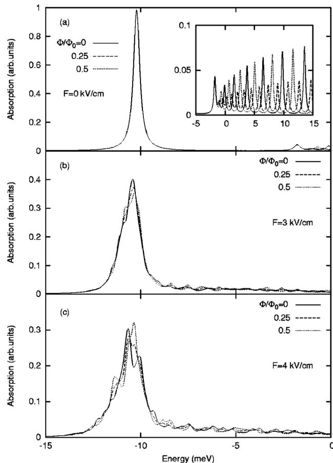
FIG. 3. Optical absorption of NR with excitonic effects for different  $F$  and  $\Phi$ . In (a), all curves are superimposed for energies below the band gap.
