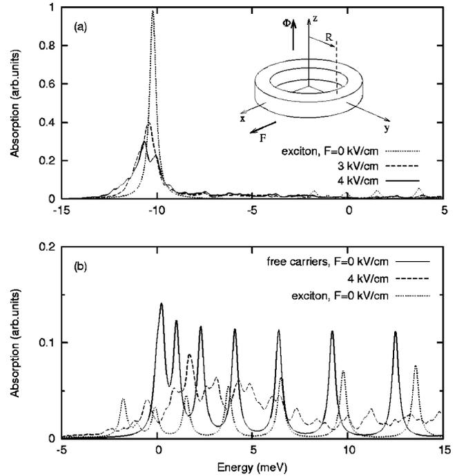
FIG. 1. Optical absorption of NR (with and without excitonic effects) for different electric-fields  $F$  in the absence of magnetic flux  $\Phi$ . Inset in (a) shows schematic of a NR in the presence of  $F$  and  $\Phi$ .
