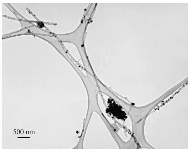
Fig. 1. Low-magnification TEM image of nodule-containing carbon nanotubes, prepared at 1000 °C (Sample 257-1).
