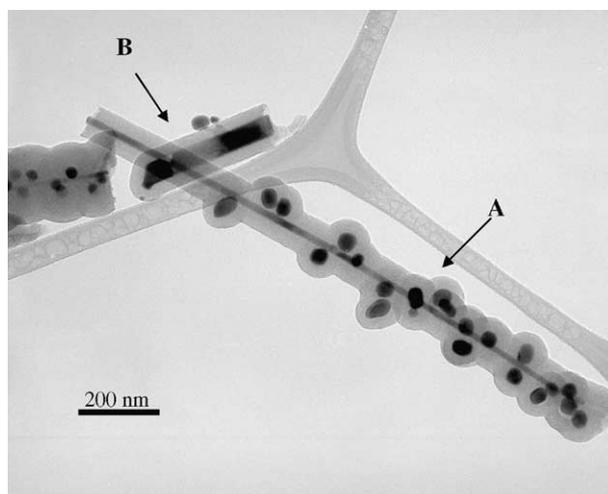
Fig. 4. TEM image of nodule-containing carbon nanotubes filled with nanowires (Sample 257-3).
