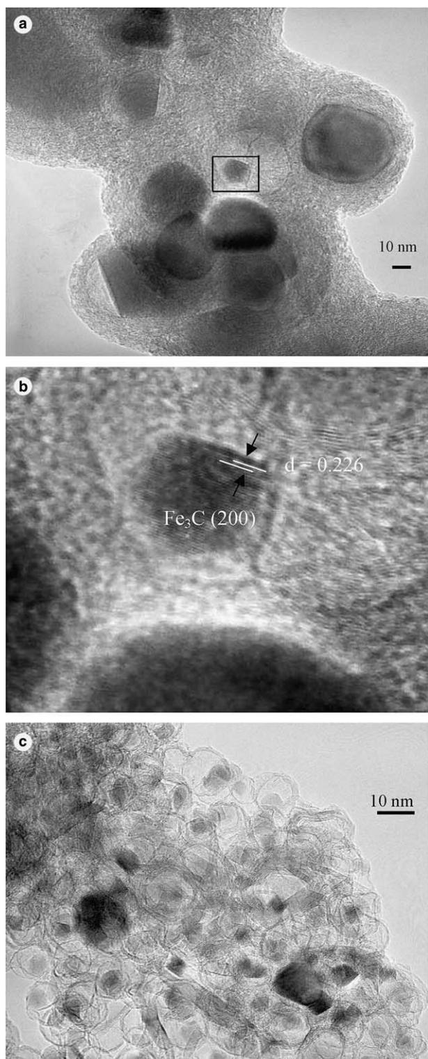
Fig. 5. (a) HRTEM micrograph of the nodule-containing carbon nanotube sample prepared at 1150 °C for 6 h (Sample 264-2). (b) A close-up of the area marked in (a). (c) A close-up of aggregated fullerene-like nanostructures. They are hollow carbon nanoparticles, some of which are partially Fe-filled.
