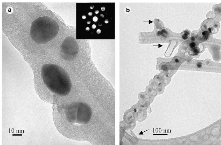
Fig. 2. (a) HRTEM image of an individual nodule-containing carbon nanotube. Inset is a selected area electron diffraction (SAED) pattern of the nodules consistent with Fe(bcc). (b) A nanotube densely covered with nodules. Arrows point to short tube branches. Both images were taken from Sample 257-1.
