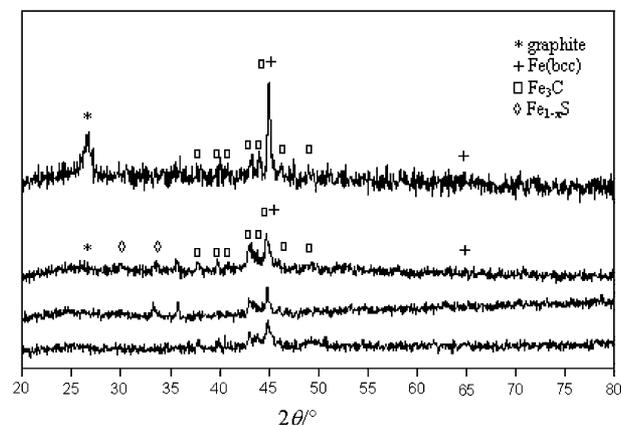
Fig. 6. XRD patterns of selected samples using different precursors. (a) Ferrocene only (Sample 164). (b) Ferrocene:thiophene ratio of 75:20; a small amount of  $\text{Fe}_{(1-x)}\text{S}$  was detected (Sample 257-1). (c) Sample in (b) treated with HCl for 14 h. (d) Ferrocene:thiophene ratio of 75:7 (Sample 257-2). From top to bottom the patterns are a, b, c and d, respectively.
