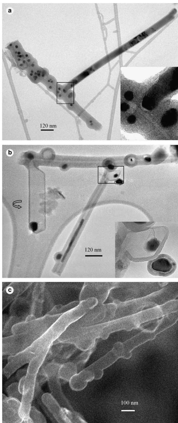
Fig. 3. (a) TEM image of an individual nodule-containing T-junction carbon nanotube. Inset is a close-up of the junction. (b) TEM image of a tube with two junctions. Inset is an HRTEM image for the right junction. (c) SEM image showing exteriors of nodule-containing and T- (or Y-) junction carbon nanotubes. All images were taken from Sample 257-3.
