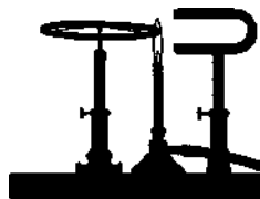
Figure 14.8 A wheel made of nickel and heated on one side will rotate in the field of a permanent magnet. At 356^\circ\text{C} , nickel loses its ferromagnetism, and then the magnet pulls in a cooler, still ferromagnetic region of the wheel. The midplane of the magnet passes through the axle of the wheel; the flame is placed in front of or behind this plane, depending on the desired sense of rotation.
