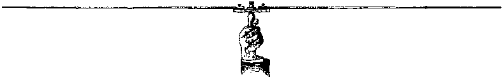
Figure 12.6 A rod-shaped electric dipole, around 1.5 m long
