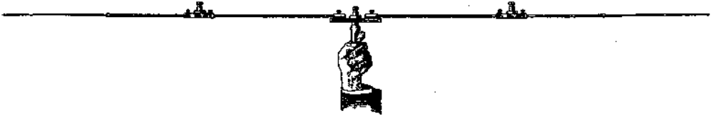
Figure 12.9 Demonstration of the sinusoidal distribution of the conduction currents along a rod-shaped dipole
