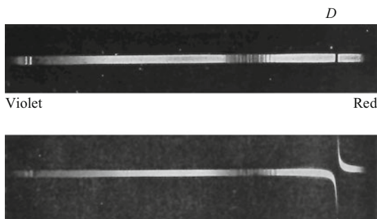
Figure 27.5 The anomalous dispersion of Na vapor, demonstrated with the apparatus in Fig. 27.4 (photographic positives). The absorption bands which are visible in addition to the D band are due to Na molecules. Because of their low particle-number densities, they have no noticeable influence on the refractive index of the vapor.
