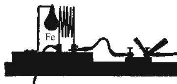
Figure 1.10 At the right is a fixed coil, at the left a coil which is free to rotate. The leads to the rotatable coil are made of woven-metal ribbons. This is a schematic of a rotating-coil instrument for measuring current or voltage, including alternating current (Sect. 10.3).
