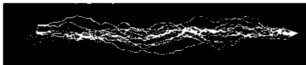
Figure 10.23 The spark discharge from an induction coil, about 40 cm long between the terminals ( S in Fig. 10.22). The coil is equipped with a mechanical interrupter, and the exposure time for this photo was 1 second.
