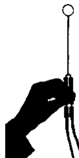
Figure 5.9 Probe coil for measuring the magnetic flux density of an electromagnet (one turn with an area of 3 \text{ cm}^2 ; this corresponds to N_J A = 3 \cdot 10^{-4} \text{ m}^2 ‘area turns’)
