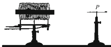
Figure 4.14 Inserting an iron core acts like an increase in the number of turns or the current (i.e. the ‘ampere-turns’) in a coil (solenoid)
