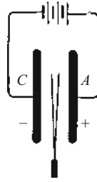
Figure 2.4 Two gold-covered quartz fibers which have spread apart (the distance between the spread fibers remains small compared to the spacing of the condenser plates A and C)
