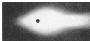
Figure 26.10 The lack of symmetry of the scattered radiation from large sulfur particles: “forward scattering”, along the direction of the primary light beam, predominates (the setup is shown in Fig. 26.9, top; the light used is unpolarized, from an incandescent lamp. This image is about 1/10 actual size).
