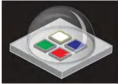
**Figure 18.1-25** A color-mixing LED comprising individually addressable red, green, and blue dies, along with a white phosphor-conversion emitter, in an SMD package capped by a 5-mm-diameter hemispherical lens. Array LEDs such as these can be electrically tuned to emit essentially any color in the gamut of human vision, including metameric white light.
