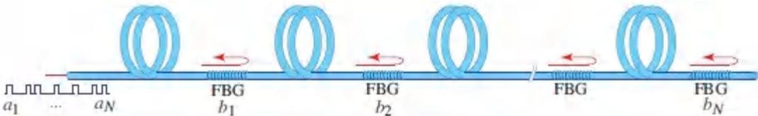
**Figure 24.3-39.** Optical correlator for recognizing the header address.
