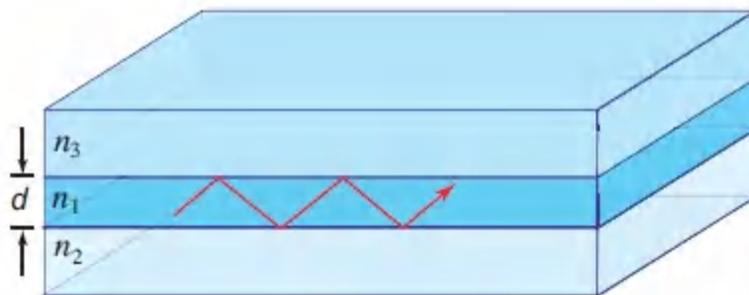
**Figure 9.2-10** Asymmetric planar waveguide.
