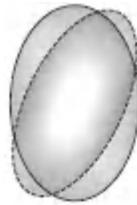
[Figure 21.2-2](#) The index ellipsoid of a crystal is modified when a steady electric field is applied.
