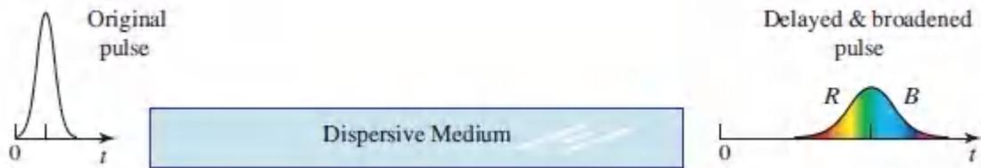
**Figure 5.5-3** A dispersive medium serves to broaden a pulse of light because the different frequency components that constitute the pulse travel at different velocities. In this illustration, the low-frequency component (long wavelength, denoted  $R$ ) travels faster than the high-frequency component (short wavelength, denoted  $B$ ) and therefore arrives earlier.
