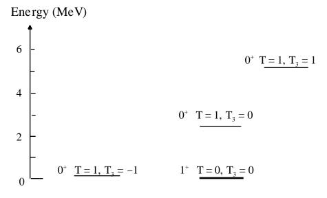
An isospin singlet (T=0) and an isospin triplet (T=1) in the A=14 system. In the absence of the coulomb interaction, the three T=1 states would be degenerate.
