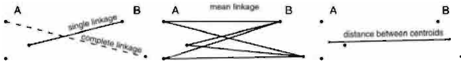
Figure 4.12 Single linkage, complete linkage (left plot), mean linkage (middle plot), and distance between centroids (right plot) for two clusters A and B.
