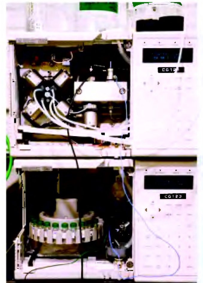
A high-performance liquid chromatography system allows geneticists to perform molecular research efficiently by automating necessary processes.
