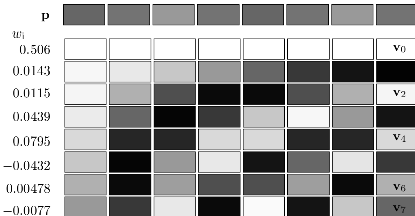
Figure 4.42: A Graphic Representation of the One-Dimensional DCT.
