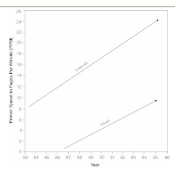
Figure 5.4 Speed Improvements in InkJet and LaserJet Printers
