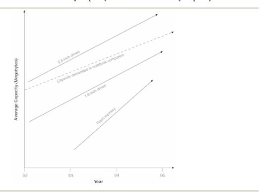
Figure 2.8 Comparison of Disk Drive Memory Capacity to Flash Card Memory Capacity
