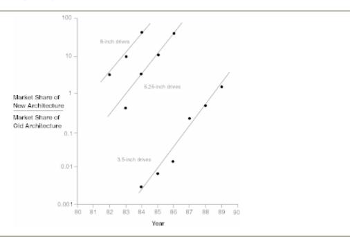
Figure 9.2 Substitution of 8-, 5.25-, and 3.5-Inch Drives of 30 to 100 MB
