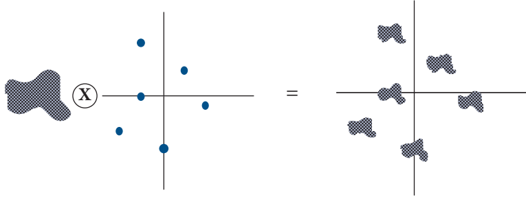
Figure 9.16 The convolution of an aperture with an array of delta functions will produce an array of identical apertures, each located at the position of one of the delta functions.
