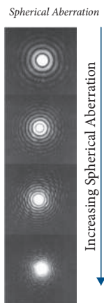
Figure 7.15 Spot diagrams of a lens as the observation point is adjusted to best focus. The aberration shown is spherical aberration.
