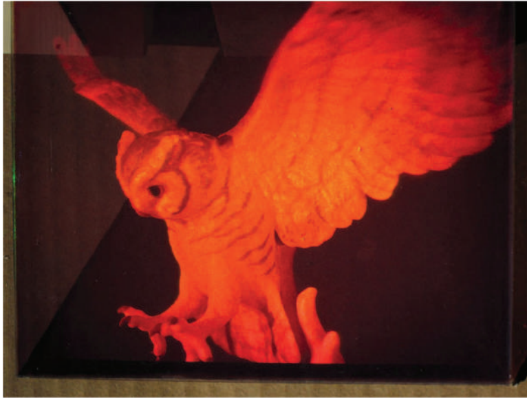
Figure 11.43 Display hologram generated by using the real image of a hologram as the object in the recording of a reflective hologram. Sunlight was used as the playback illumination.
