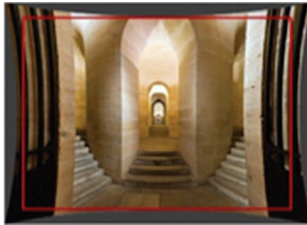
Figure 7.27 Pincushion distortion can be seen as the edges of the walls in the figure curve outward at the top and bottom. Pincushion is associated with positive distortion, displayed in graph at the left.
