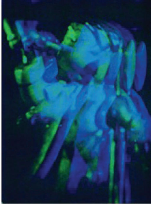
Figure 9.17 Hologram of Hummel figurine (Hear Ye! Hear Ye!) reconstructed using three different wavelengths. The wavelength sensitivity is due to diffraction by photographically recorded interference fringes. (Hologram courtesy of N. George.)
