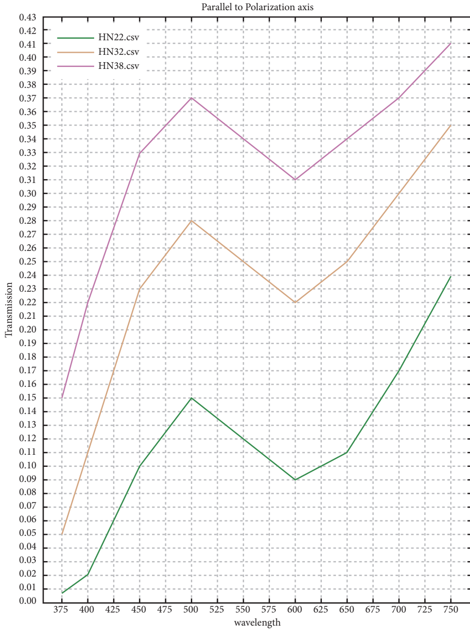
Figure 5.7 The transmission of light polarized parallel to the Polaroid axis. Two different grades of H-sheet are shown. These curves should be compared to those shown in Figure 5.8.
