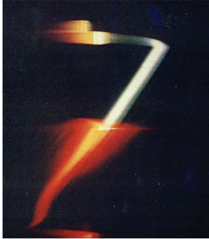
Figure 3.23 Blue laser light is shown propagating in xylene (above) and water (below). The water contains the dye Rhodamine 6G in solution. The red Rhodamine dye absorbs the blue light and the blue beam rapidly decays to 0. Some of the energy absorbed by the dye is re-emitted in the yellow to red region of the spectrum. This re-emitted light caused the diffuse appearance of the light as it propagates in the water because the dye molecules are moving in the solution.
