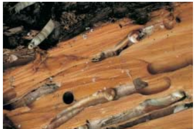
Shipworms ( Bankia setacea ) in fallen piling. Without being detected, shipworms can drill through lumber until it resembles a honeycomb and is rendered unfit for use. (Photo by Gary Gibson/Photo Researchers, Inc. Reproduced by permission.)
