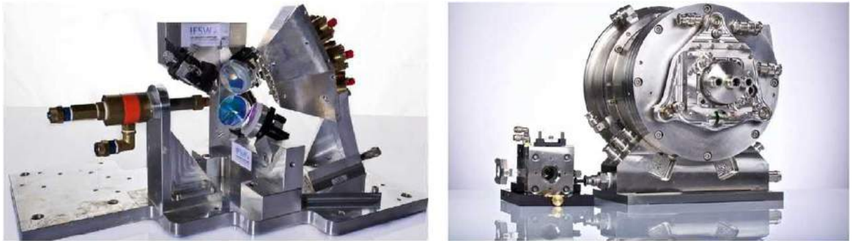
Fig. 4 Left: one of the first thin-disk laser (TDL) setups, demonstrated an output power of 100 W. This setup provides eight passes of the pump power radiation through the thin disk (courtesy of IFSW). Right picture shows two disk modules: the smaller one is designed for 1 kW pump power and the larger one – for 30 kW. Both modules provide 24 or 48 passes of pump radiation through the laser disk, depending on the pump beam quality. Dausinger + Giesen GmbH.
