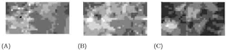
Fig. 4. The dividing maps of viewpoint space observed using range sensor are showed. y axis is latitude, which is \eta = 0^\circ \sim 180^\circ , and x axis is longitude, which is \zeta = 0^\circ \sim 360^\circ . ((A) t=20 , (B) t=90 , (C) t=270 )
