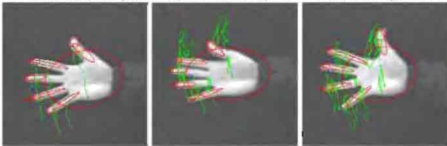
The behaviour of the qualitative feature hierarchy tracker under semi-rigid motion
