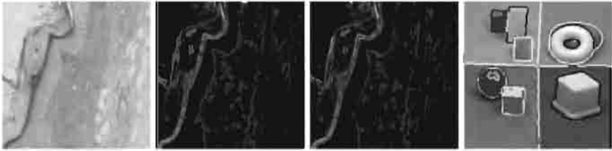
Fig. 1. Illumination invariant edges for epithelial tissue (a) visualized by transmission light microscopy. Edges N_{\lambda w} = \sqrt{N_{\lambda x}^2 + N_{\lambda y}^2} are shown for (b) a white illumination (halogen 3400K), and (c) a reddish illumination (halogen 2450K). Despite the different illuminants, edge strength is comparable. Figure d shows zero crossing detection in an image of colored objects. In white the N_{\lambda w w} crossings (bluish-yellow edges), in black the N_{\lambda \lambda w w} crossings (reddish-green edges).
