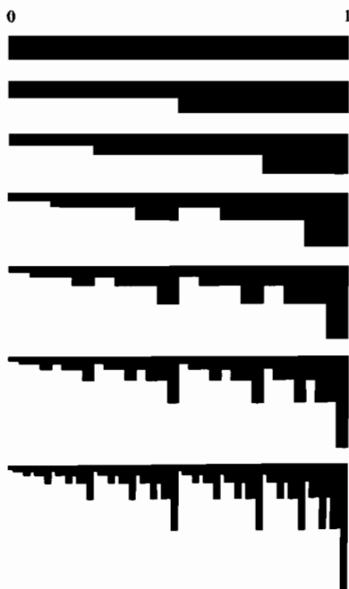
Figure 10.1 Construction of the self-similar measure of Proposition 10.4 by repeated subdivision of measure in the ratio \frac{1}{3} : \frac{2}{3} , that is with p = \frac{1}{3}
