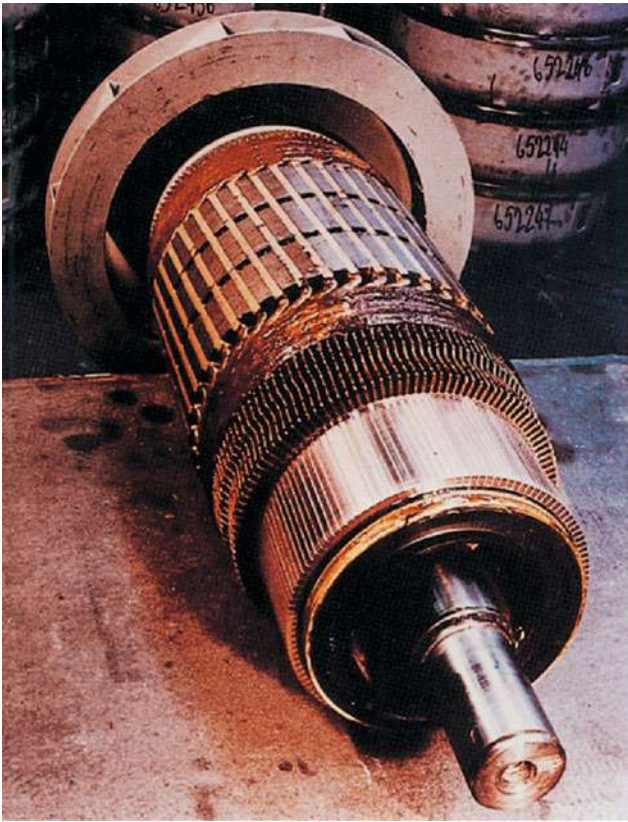
Fig. 5.6 Rotating part of a dc-motor with commutator, armature windings and fan propeller, (with kind permission of Siemens AG)
