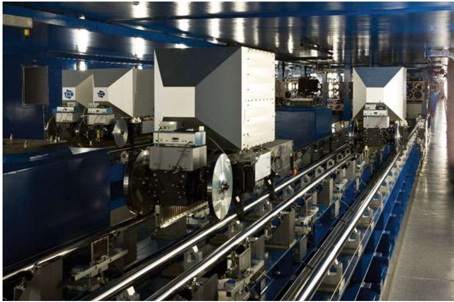
Fig. 12.13 Part of the interferometric path with a retro-reflecting mirror mounted on a wagon which moves smoothly on a track (ESO observatory on the Paranal in Chile)
