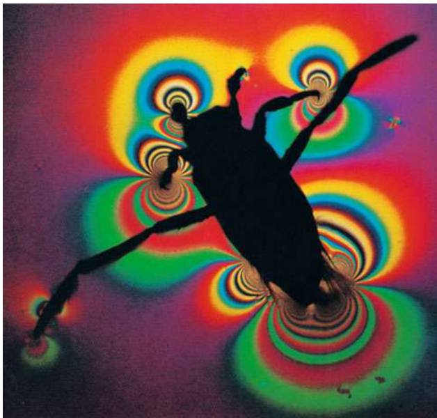
Fig. 8.47 Wird 8.54x Water runner on a water surface. The interference fringes around the legs indicate the deformation of the water surface, which depend on the balance between weight of the animal and the surface tension of the water. From Francon and Malik (1971)
