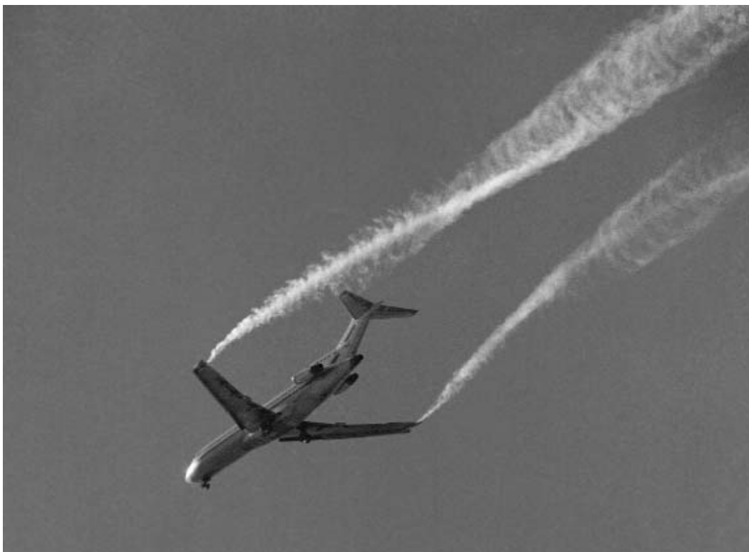
Figure 7.9: Vortices trailing from the wingtips of a Boeing 727.
