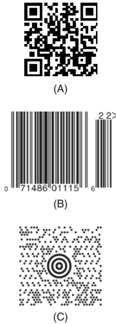
Figure 12-3. (A) Two-dimensional QR code for this book's website ( http://www.understandinglasers.com ) (B) A one-dimensional UPC symbol from a magazine. (C) Maxicode for this book's website ( http://www.understandinglasers.com ).
