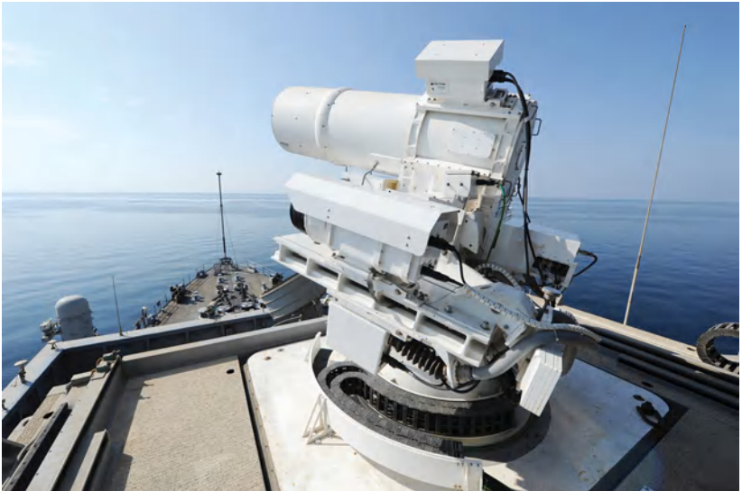
Figure 13-9. The Navy LaWS experimental laser weapon, installed on the USS Ponce in the Persian Gulf in November 2014. This 30-kW system focused light from six industrial fiber laser to shoot down drones and detonate explosives on small boats. Color in electronic edition. (U.S. Navy photo by John F. Williams)
