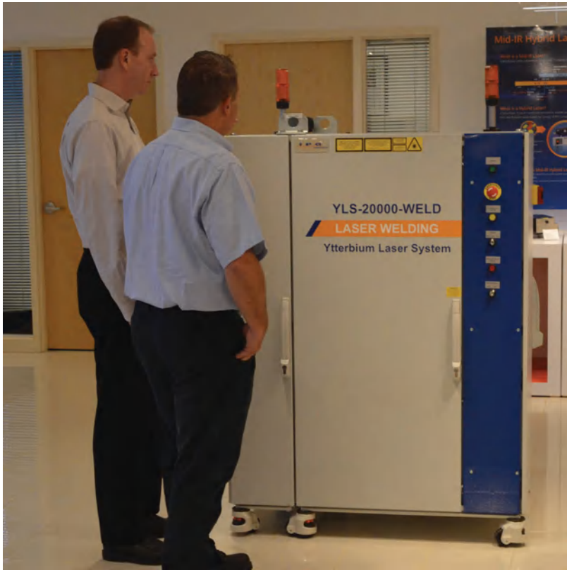
Figure 9-2. A commercial multimode ytterbium-doped fiber laser that generates a steady 20-kilowatt beam for welding metals weighs in at about 600 kilograms and is comparable in size to a family refrigerator. The fiber architecture makes it remarkably compact for such a powerful laser. Photo by Alexei Markevitch, Courtesy of IPG Photonics.
