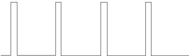
Figure 6-2. A quasi-continuous laser emits for short intervals than switches off for lower intervals to dissipate waste heat. Typical diode arrays emit individual pulses lasting 0.05 to 50 milliseconds.
