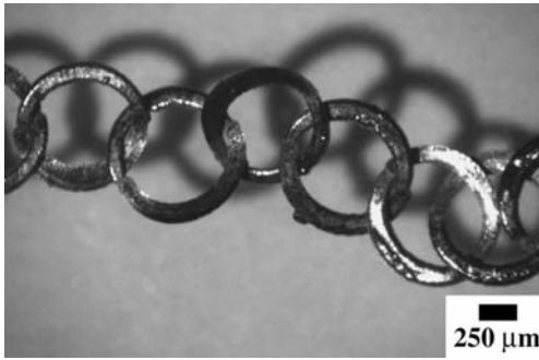
Figure 3.11 Optical micrograph of a free-jointed nickel chain formed by the process shown in Figure 3.10 [33]. The final thickness of the nickel was about 50 \mu\text{m} .
