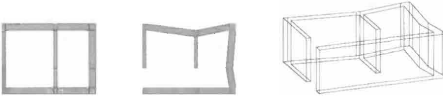
Figure 7.28 (a) Polygon generated by a quadArray primitive (b) Polygon generated by a quadArray primitive (c) Extruded solid
