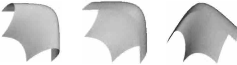
Figure 12.18 Some pictures of a new surface interpolating the same Hermite curves with constant oblique tangent vectors.
