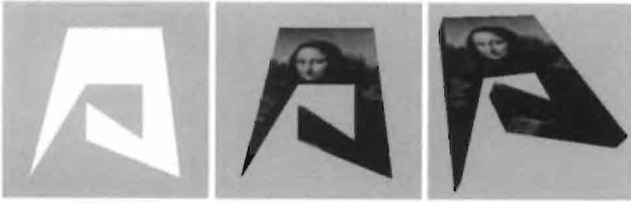
Figure 10.48 (a) Polygon generated by a triangleStrip (b) Texture mapping on polygon; (c) polygon extrusion followed by texture mapping
