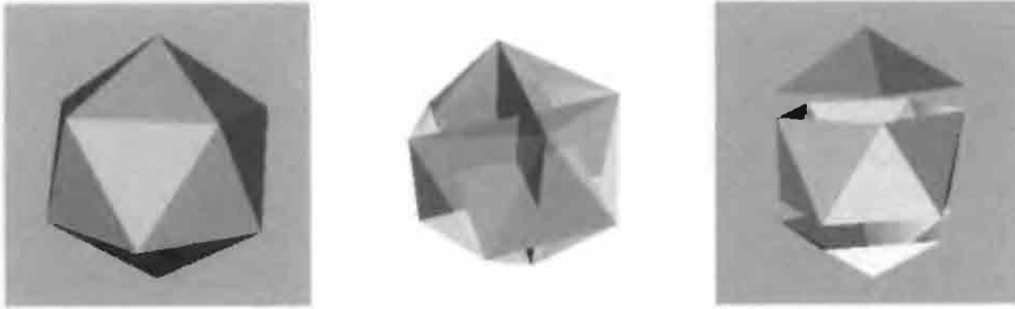
Figure 4.20 (a) Icosahedron (b) Generation of icosahedron as JOIN of three orthogonal rectangles with sides in the golden ratio (c) Layered structure of icosahedron
