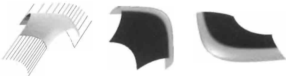
Figure 5.17 Gauss curvature field: (a) surface generated by Hermite's transfinite interpolation of two curves and two (constant) vector fields (b) subset of negative Gauss curvature (c) subset of positive Gauss curvature
