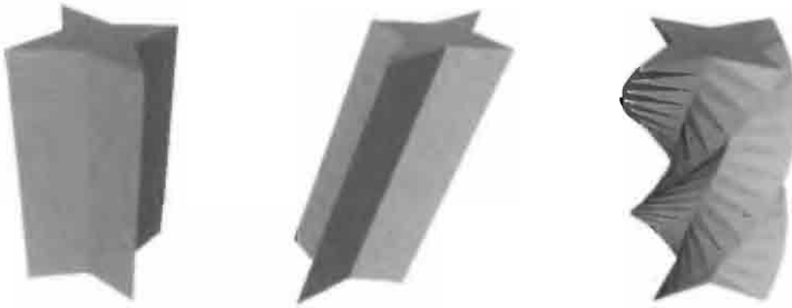
Figure 15.17 3D polyhedral encoding of a degree of freedom of a 2D object: (a) straight extrusion (independence on parameter) (b) linear extrusion (translational DOF) (c) screw extrusion (rotational DOF)
