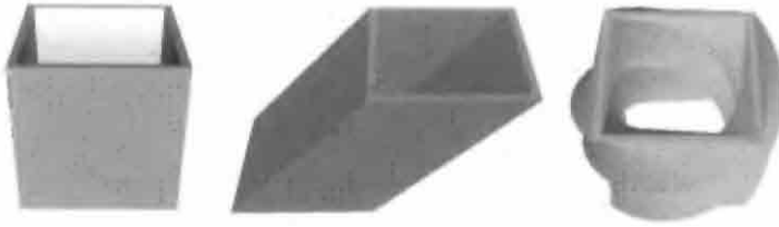
Figure 15.18 Encoding of a DOF via straight, linear and screw extrusions produced by EX, LEX and SEX operators
