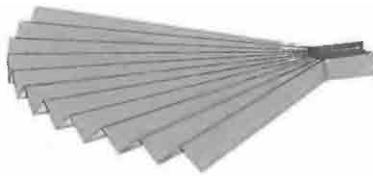
Figure 7.18 Interesting use of the QUADMESH primitive: the fan object
