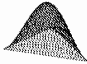
Figure 6.19 Nodal basis of the cubic Hermite element; the bubble function \varphi_t^b .
