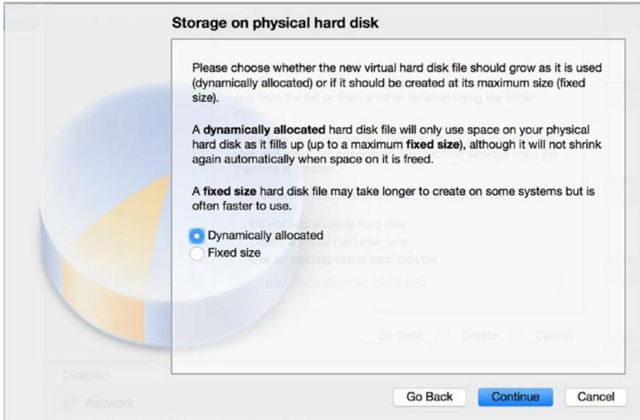
**Figure 3-6.** Dynamically allocating disk
