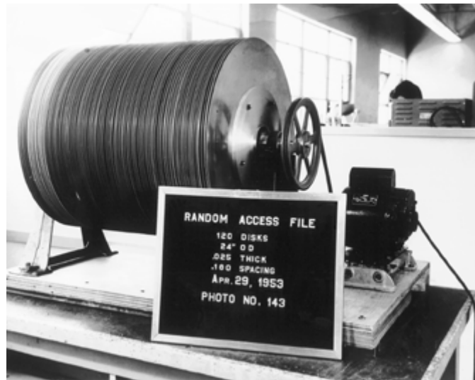
Figure 1.2 The First Disk Drive, Developed by IBM
