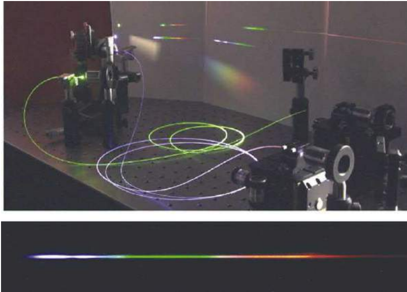
Fig. 9 Photograph of fiber generating the supercontinuum. The bottom photo shows the continuum after passing through a prism.
