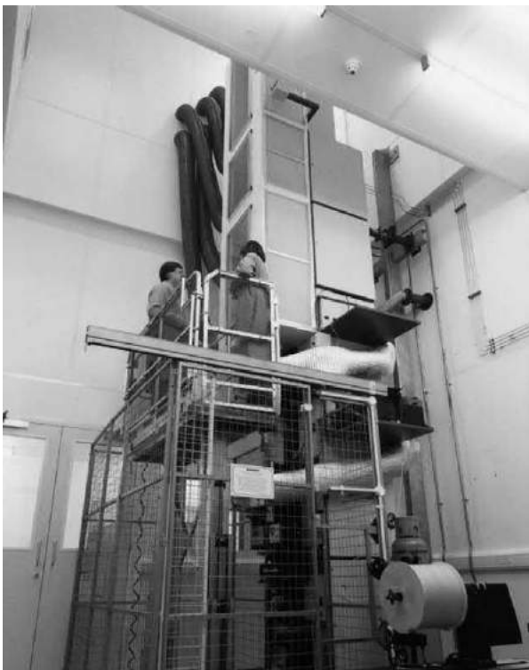
Fig. 5 A commercial scale optical fiber drawing tower.
