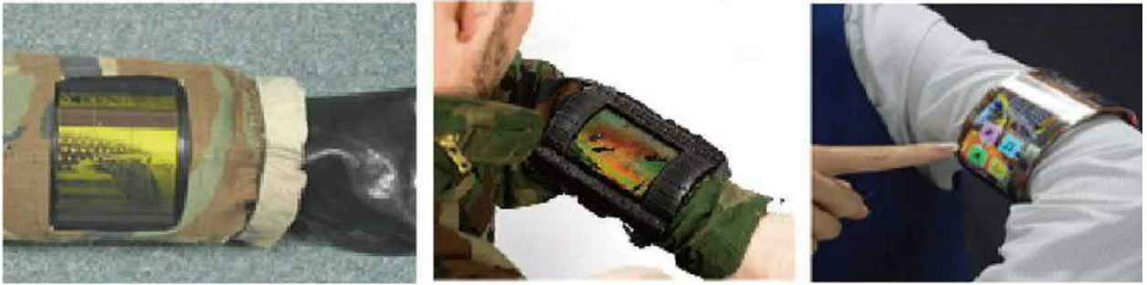
Fig. 4 The prototypes of the wearable-display wrist unit. Reproduced from Ma, R.Q., Rajan, K., Silvernail, J., et al. , 2010. Wearable 4-in. QVGA full-color-video flexible AMOLEDs for rugged applications. Journal of the Society for Information Display 18, 50–56; Tajima, R., Miwa, T., Oguni, T., et al. , 2014. Truly wearable display comprised of a flexible battery, flexible display panel, and flexible printed circuit. Journal of the Society for Information Display 22, 237–244.
