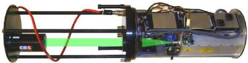
Fig. 6 Internal layout of eHolocam showing the laser, power supply and computer on the right and the smaller CMOS housing on the left.
