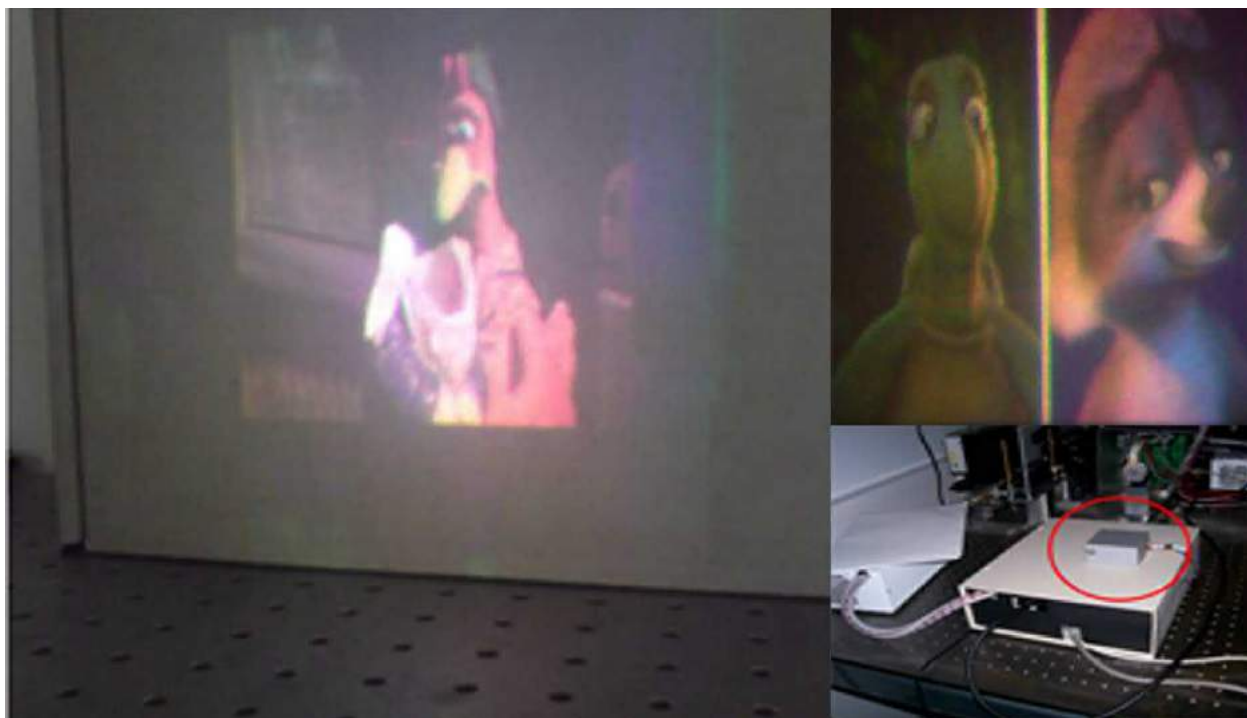
Fig. 12 A handheld holographic video projector with real-time CGHs developed in CAPE of Cambridge University and made by Alps Electric in Japan. Reproduced from SPIE, 2017. Available at: http://spie.org/newsroom/1015-projection-display-using-computer-generated-phase-screens?highlight=x2408&ArticleID=x20068 (accessed 21.05.17).
