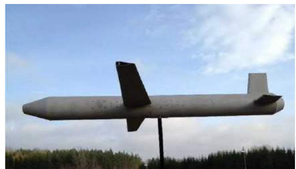
Fig. 16 Measurement with the photon-counting system on the UAV mock-up at 1.3 km distance. In the middle a waveform contains the target and terrain background. Right shows the resulting intensity of each pixel (approximately 15 cm square) in the photon-counting system when it was scanned over the target. Reproduced from Steinvall, O., Tuldahl, M. 2016. Laser range profiling for small target recognition. Optical Engineering 56 (3), 031206.
