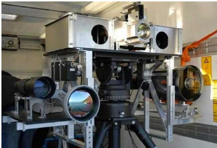
Fig. 9 Marine target sensing testbed with 1550-nm laser and two receivers. Below is optics for two cameras and Celestron telescope. Reproduced from Steinvall, O., Tuldahl, M., 2017. Laser range profiling for small target recognition. Opt. Eng. 56 (3), 031206.
