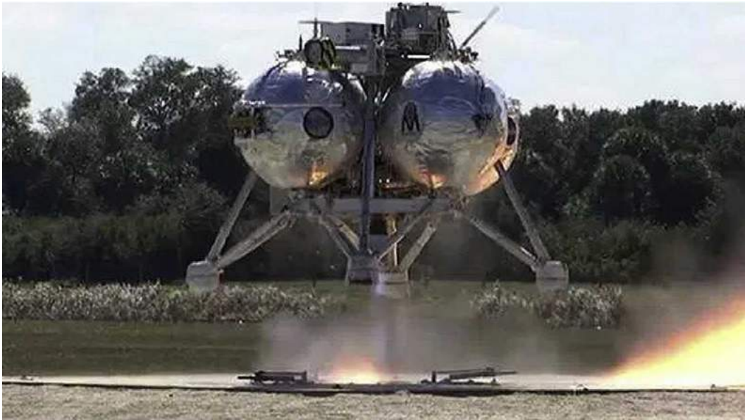
Fig. 12 Morpheus lander in the last moments of landing with ALHAT laser radar instruments. Reproduced from Morpheus lander. Available at: https://morpheuslander.jsc.nasa.gov .
