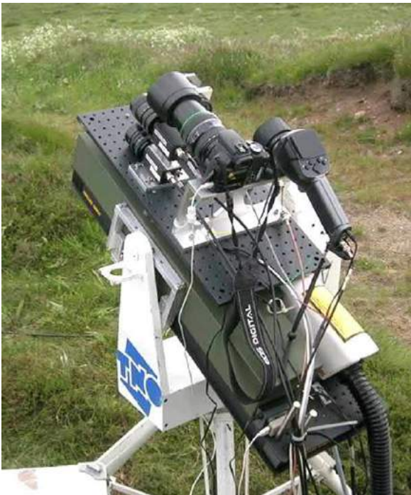
Fig. 6 Laser Range Profiler for the MCG/8 trial. Reproduced from Heuvel van den, J.C., Pace, P., Bekman, H.H., et al. , 2008. Experimental validation of ship identification with a laser range profiler. Proc. SPIE 6950, 69500V.
