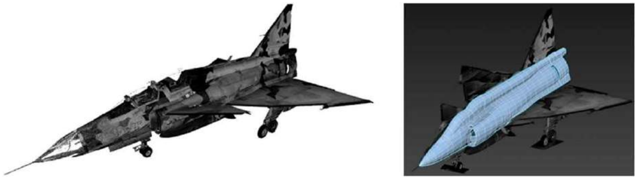
Fig. 4 Left: a point cloud model of aircraft SK37 Viggen using the Riegl VZ-400 laser scanner. Right: the polygon model built with the point cloud as a reference. Images FOI.
