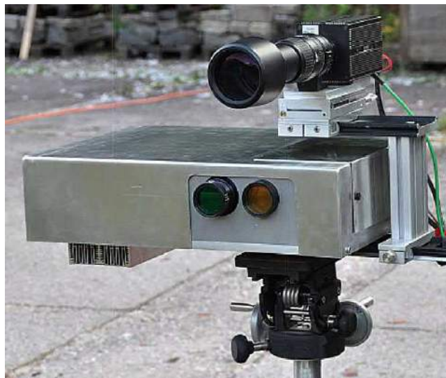
Fig. 15 SAVIS laser Doppler vibrometer. Reproduced from Lutzmann, P., Göhler, B., Putten, F., Hill, C.A., 2011. Laser vibration sensing: Overview and applications. Proc. SPIE 8186, 818602.
