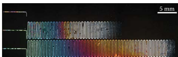
FIGURE 7.4 Correlations between the length of the bright LC regions and the concentration of anti-IgG. From the top, the concentration of anti-IgG was 0.02, 0.05, and 0.08 mg/mL, respectively.
