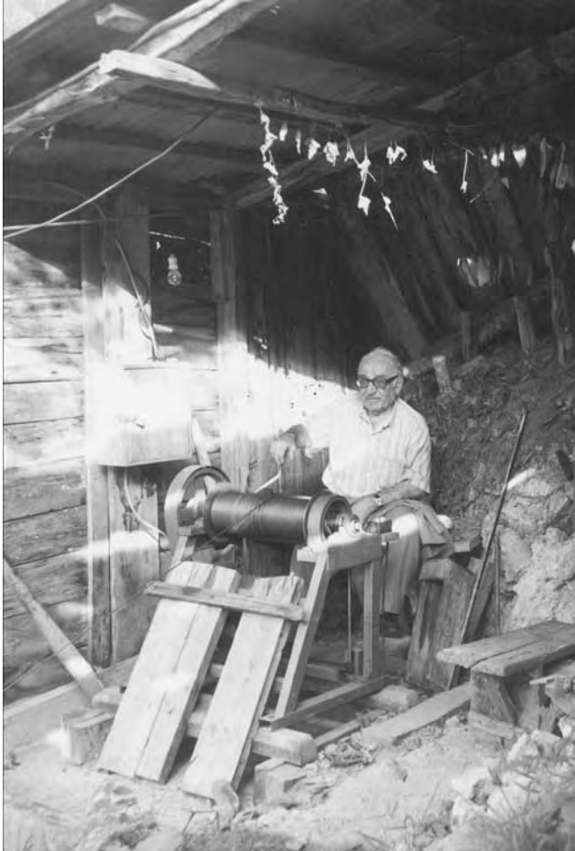
Figure 8.6 Control room of a steel cable lift ( teleferik ) in the Makrevis (Konaklar) mahalle. These systems are used to transport heavy loads from roads on valley floors to houses which have no motor vehicle access.
