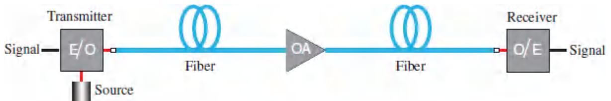
**[Figure 25.0-1](#)** Schematic of an optical fiber communication system. An electrical signal is converted into an optical signal (E/O) by modulating an optical source. The optical signal is transmitted through the fiber to the receiver, where it is converted back into an electrical signal via a photodetector and demodulator (O/E). For long links, optical amplifiers (OAs) can be used to boost the attenuated optical signal.
