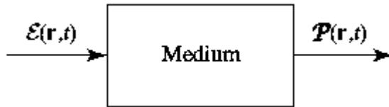
**Figure 5.2-1** In response to an applied electric field  $\epsilon$ , the dielectric medium creates a polarization density  $\mathcal{P}$ .
