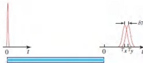
**Figure 10.3-7** Differential group delay (DGD) associated with polarization mode dispersion (PMD).
