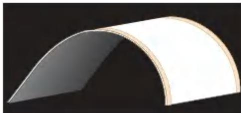
**[Figure 18.1-28](#)** A 1/4-mm-thick white OLED light panel that generates metameric white light with a luminous flux  $P_v = 75$  lm, a luminous efficacy  $\eta_v = 60$  lm/W, a CCT = 3000° K, and a CRI = 90. It has a life span of some 40 000 hours. Such panels offer large-area homogeneous illumination.
