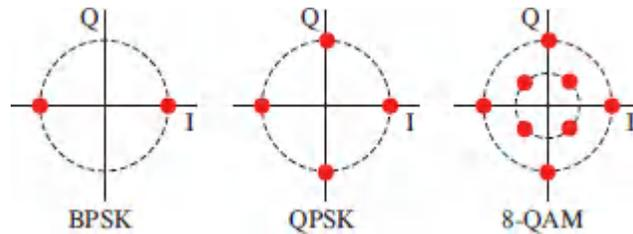
**Figure 25.3-5** Constellations for BPSK (1 bit), QPSK (2 bits; also called 4-QAM), and 8-QAM (4 bits). The symbols I and Q denote the in-phase and quadrature components of the complex amplitude, which are the real and imaginary components, respectively.
