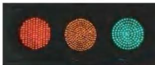
**Figure 18.1-17** LED traffic signal based on III–V materials.
