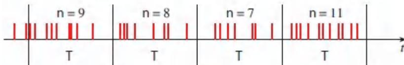
[Figure 13.2-4](#). Random arrival of photons for a coherent light source of power  $P$ . Consecutive counting times of duration  $\mathcal{T}$  are indicated. Though the optical power is constant, the photon number  $n$  observed in each counting time is random.
