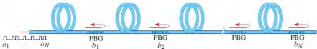
**Figure 24.3-39.** Optical correlator for recognizing the header address.
