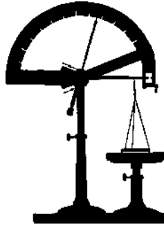
Figure 9.18 The measurement of the specific surface energy using a spiral spring balance. A numerical example for water: ring diameter 5 cm, circumference 2l = 0.31 m, F = 2.26 \cdot 10^{-2} N, \zeta = 0.072 W s/m 2 .
