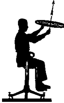
Figure 6.17 The conservation of angular momentum. The arrows represent the angular momenta of the wheel and the experimenter. (At small angular velocities, the motion is disturbed by the residual friction.) (Video 6.3)
