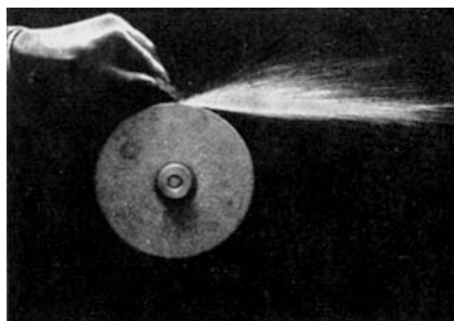
Figure 4.6 A grinding wheel, spraying sparks C4.3
