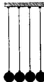
Figure 5.18 The demonstration of elastic collisions between two objects of the same mass. The balls are hung by two threads (“bifilar suspension”), so that they can move freely from left to right (but not forward or backward). (Video 5.4)
