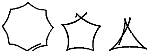
Figure 6.40 Left: The weak nutation of a suspended top, the approach to pseudo-regular precession; center and right: increasing nutation as the angular momentum of the top decreases (photo negatives)
