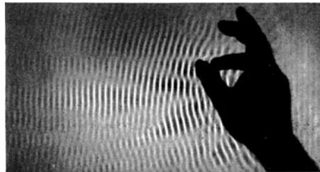
Figure 12.49 The acoustic replica method makes visible the interference field of high-frequency sound waves in front of a hand which is reflecting them (a ‘snapshot’, i.e. the hand did not move during the exposure time)
