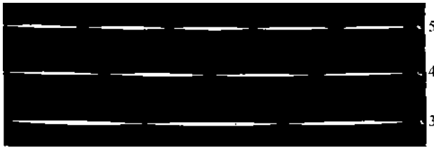
Figure 11.27 The third to the fifth torsional oscillation modes of a 1 m long and 3 cm wide stretched rubber band. The holder at one end is turned back and forth by an eccentric on an axis parallel to the long axis of the band; angles of a few degrees are sufficient.
