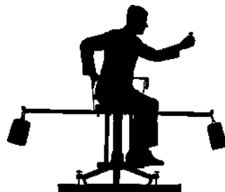
Figure 7.16 A swivel chair with a large moment of inertia for demonstrating CORIOLIS forces. The heavy weights hanging at the sides can also be conveniently used for the experiments shown in Figs. 7.7, 7.11, 7.13 and 7.15 C7.9
