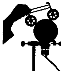
Figure 6.37 A model bicycle is “spun up” by pressing its wheels onto a rapidly rotating disk on the shaft of an electric motor (Video 6.12)
