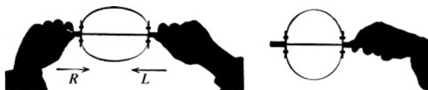
Figure 3.4 Deformation of a circular spring. In the center of the spring is a guide rod. This simple apparatus will be used later for demonstration experiments as an uncalibrated force meter.
