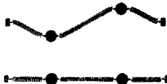
Figure 11.18 Transverse vibrations of two coupled elementary oscillators; the balls vibrate with a 180^\circ phase shift, i.e. in opposite directions (stopped-motion images)
