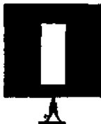
Figure 12.61 The diffraction slit used in Fig. 12.60; its width is B = 11.5 cm
