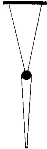
Figure 11.53 Two coupled gravity pendulums, hung in a bifilar arrangement, with inertial elements of very different mass. They can swing in a plane perpendicular to the page. (Video 11.8)
