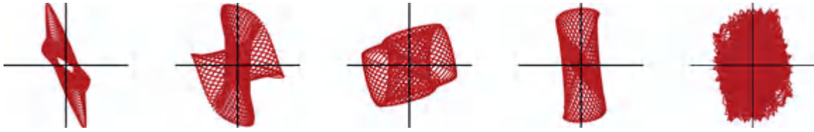
Figure 3.11 The randomly evolving polarization ellipse for the state of Figure 3.10 (right) in four (left, second, third, and fourth) consecutive time periods of equal duration. (Right) The polarization ellipse graphed over a longer period of time shows it approaching a random unpolarized distribution.
