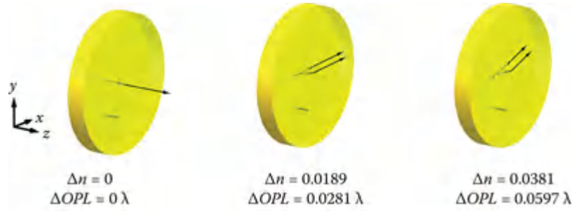
Figure 21.31 Three incident rays at 0.5 \mu\text{m} with incident angles 0^\circ , 30^\circ , and 45^\circ pass through a quarter wave C-plate and experience different birefringence \Delta n and \Delta OPL . An exaggerated thickness is shown to demonstrate the ray splitting.
