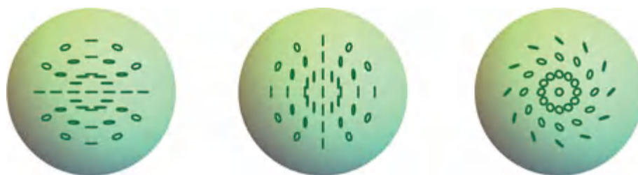
Figure 21.35 The exiting polarization ellipses from a 6.3 \mu\text{m} C-plate for horizontally (left), vertically (middle), and circular (right) polarized spherical incident wavefronts.
