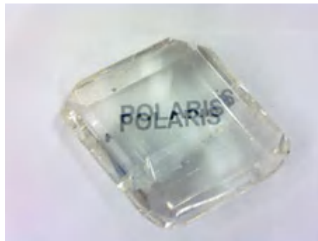
Figure 21.1 Imaging doubling through a piece of calcite.
