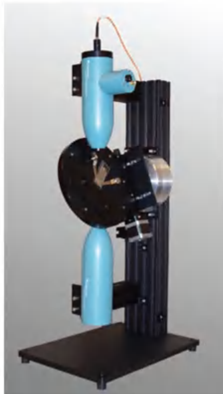
Figure 1.13 (Top) A Mueller matrix imaging polarimeter illuminates and measures a sample with many combinations of illuminating polarizers and analyzing polarizers to measure the Mueller matrix, diattenuation, retardance, and depolarization of samples. This particular Mueller matrix polarimeter illuminates the sample through a linear polarizer and a retarder that steps in angle. The light interacts with a sample and exits with its polarization state changed. The light may reflect from, transmit through, diffract from, or scatter from a sample depending on the measurement. This change is analyzed by a retarder that steps in angle and a linear polarizer
