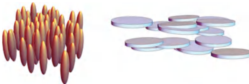
Figure 24.4 Schematics for nematic molecules (left) and discotic molecules (right).
