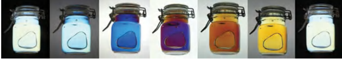
Figure 19.10 Light propagating through corn syrup (concentrated sugar water solution) in a polariscope. The angle between the polarizer axes rotates 180^\circ from the left figure to the right figure. The polarizer axes are crossed in the left-hand image, parallel in the middle image, and crossed again in the right-hand image. The colors arise from the dispersion of the polarization state, being rotated by a larger angle in the blue and a smaller angle in the red. For this specific jar, the blue–purple light has been rotated by more than 180^\circ while the red light has been rotated by about 135^\circ .
