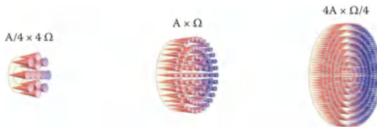
Figure 10.20 Three beams of light with the same etendue \Xi = A \Omega . (Center) An area A where the rays from each point fill a solid angle \Omega . (Left) An area A/4 where the rays from each point fill 4 \Omega . (Right) An area 4A where the rays from each point fill \Omega/4 .
