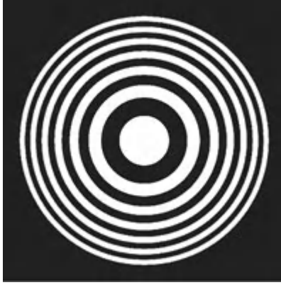
Figure 23.4 Fresnel zone patterns where white has a transmission of 1 and black has 0 transmission.
