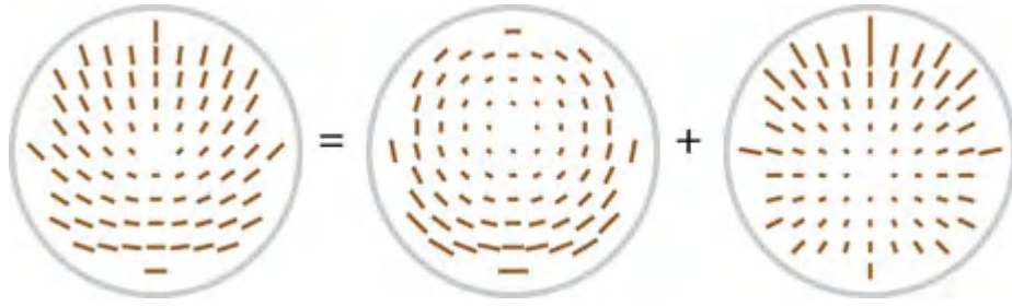
Figure 15.15 Pure polarization tilt can be generated from two equal but opposite polarization defocus contributions, one shifted up, the other shifted down.
