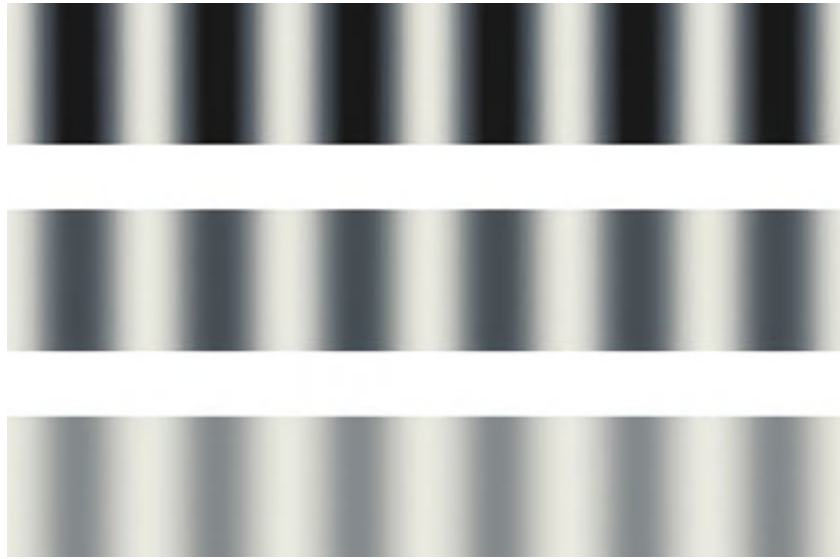
Figure 4.7 Fringe patterns between two beams with identical polarization states obtained by interfering two beams of equal flux, P_1/P_2 = 1 , (top) yielding a fringe visibility of one, (middle) P_1/P_2 = 1/3 with a visibility of 0.5, and (bottom) P_1/P_2 = 9/11 with a visibility of 0.1.
