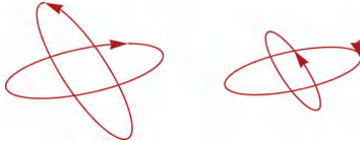
Figure 5.17 Normalized incident eigenpolarizations (left) and exiting eigenpolarizations (right). Note that major axes are not orthogonal; hence, eigenpolarizations are not orthogonal. Both diattenuation and retardance are present.
