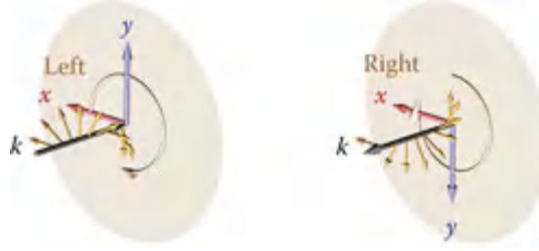
Figure 8.12 In a right-handed coordinate system containing \mathbf{k} , left circular polarization always reflects into right circular polarization at normal incidence from an isotropic interface.
