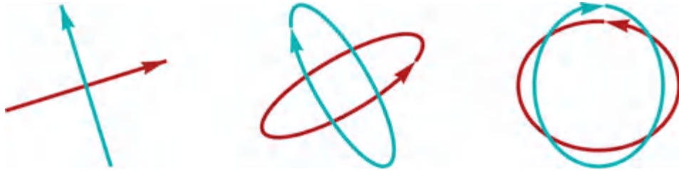
Figure 2.16 Orthogonal polarization states have major axes 90^\circ apart, opposite helicities, and equal ellipticity magnitudes.
