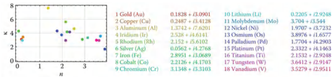
Figure 8.26 Complex refractive indices of common metals at 633 nm contain a real part n and an imaginary part \kappa .
