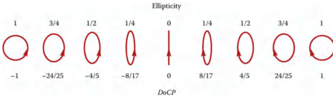
Figure 3.14 Polarization ellipses with varying ellipticity and degree of circular polarization.
