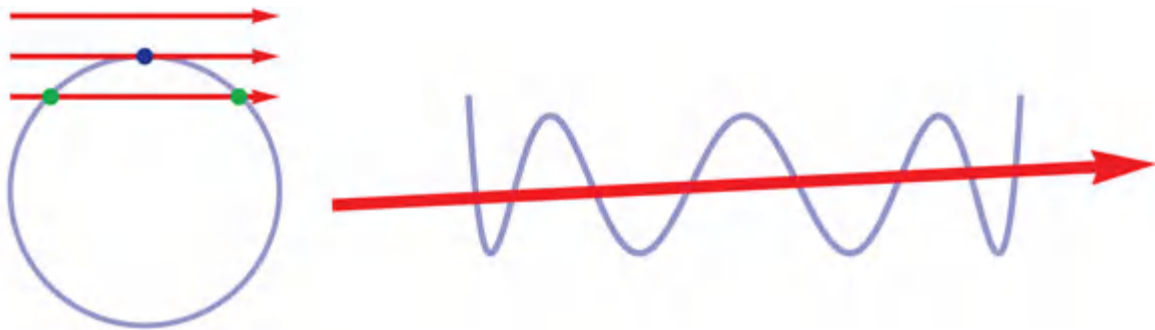
Figure 10.24 (Left) A ray intercepting a spherical surface can have two ray intercepts (green), one (blue), or none. (Right) More complex surfaces, such as aspheric surfaces, can have many ray intercepts.
