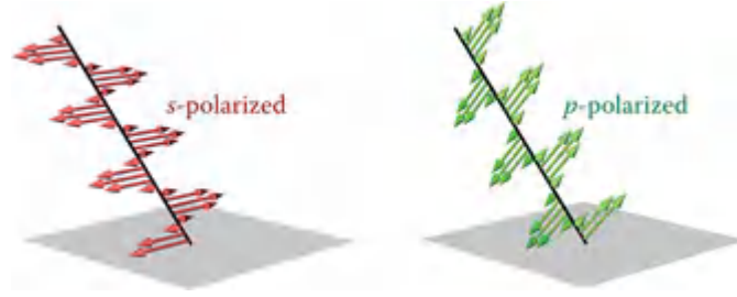
Figure 8.4 The electric fields for s - and p -polarized components of a beam of light incident on an interface. (Left) s -component perpendicular to the plane of incidence. (Right) p -component in the plane of incidence. The s -component lies on the surface while the p -component has a component into the surface.
