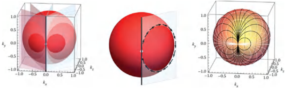
Figure 11.12 A set of circles depicting the orientation of the double pole basis vectors around the sphere is constructed by first placing a line (black) through the double pole (center of white spot) tangent to the unit propagation sphere. (Left) A series of planes are constructed through the line intersecting the unit propagation sphere ( k_x, k_y, k_z ) generating a set of circles of varying sizes that all intersect at the double pole. (Middle) The orientation of the \hat{\mathbf{y}}_{loc} basis vector is shown aligned with one of the circles. (Right) The orientation of the basis vectors over the sphere is shown for \hat{\mathbf{x}}_{loc} in white and \hat{\mathbf{y}}_{loc} in black. These are the equivalent of the lines of constant latitude and lines of constant longitude in the dipole coordinate system.
