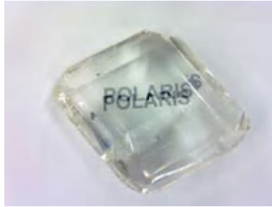
Figure 19.13 Double refraction through a calcite rhomb.
