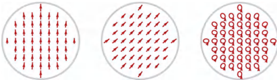
Figure 1.34 The effect of the diattenuation aberration of Figure 1.33 on incident (left) 90^\circ linear, (center) 45^\circ linear, and (right) left circularly polarized beams.
