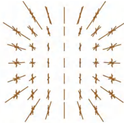
The diattenuation components for an off-axis beam through a cell phone lens, surface by surface, overlapped in the exit pupil.
