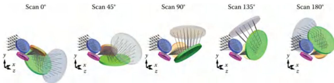
Figure 12.34 Ray trace figures showing a converging beam reflecting from M1 (blue), M2 (magenta), M3 (yellow), then M4 (green), and finally reaching a detector (gray). M1 – M2 assembly is fixed, while the M3 – M4 assembly scans about the x -axis.
