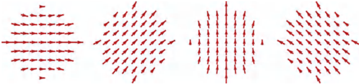
Figure 15.8 The transmitted polarization ellipse map for the diattenuation map of Figure 15.7 when, from left to right, 0^\circ , 45^\circ , 90^\circ , and 135^\circ linearly polarized light is incident. Diattenuation magnitude is 0.3 for the marginal ray in this example.
