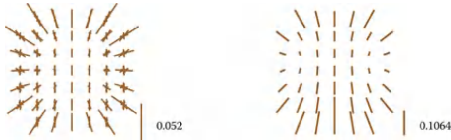
Figure 10.5 (Left) The diattenuation maps for each surface from Figure 10.4 are aligned and overlaid. (Right) The cumulative diattenuation is displayed at the exit pupil of the cell phone lens.
