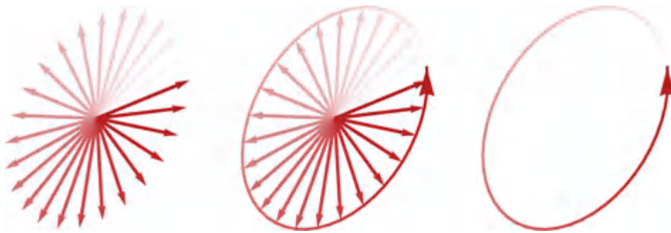
Figure 1.4 (Left) The polarization ellipse for an elliptical polarization state is the ellipse drawn by the tip of the electric field vector during one period. (Middle) The electric field as a function of time is shown with the bounding ellipse. (Right) Usually, just the ellipse is drawn to indicate the polarization state. The location of the arrow indicates the phase of the wave.
