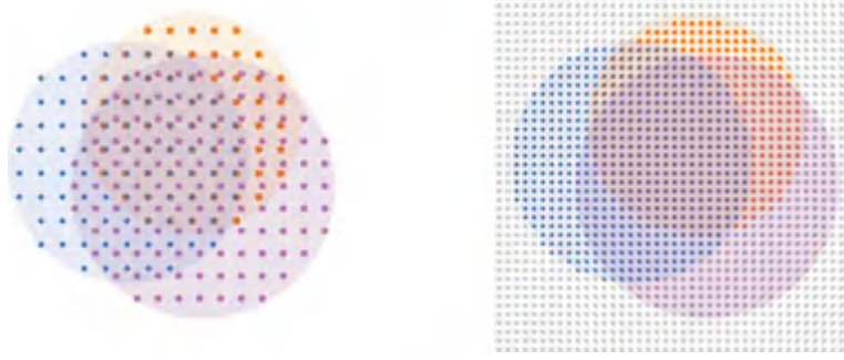
Figure 20.16 Three grids of rays corresponding to three modes reach a 2D plane. (Left) The location of the rays is shown as dots. (Right) The ray data are resampled in a regular grid with zero values (gray dots) outside the region of the three beams.
