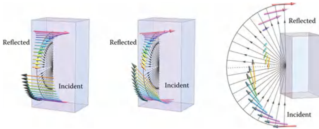
Figure 8.19 External reflection for the incident s -polarized states (left), 45^\circ polarization states (center), and p -polarized states (right) as angles of incidence change from 7^\circ to 88^\circ near grazing incidence. Since the p -polarization figures would overlap for different angles of incidence, each incident and reflected pair has been spatially translated for better visualization. The blue arrow indicates the reflected electric field at Brewster's angle. Each incident electric field vector (black arrowhead) and corresponding reflected electric field vector (colored arrowhead) pair is plotted in the same color. The arrows represent the oscillations of the electric field vector in time. The length of the arrow represents the amplitude of the electric field vector.
