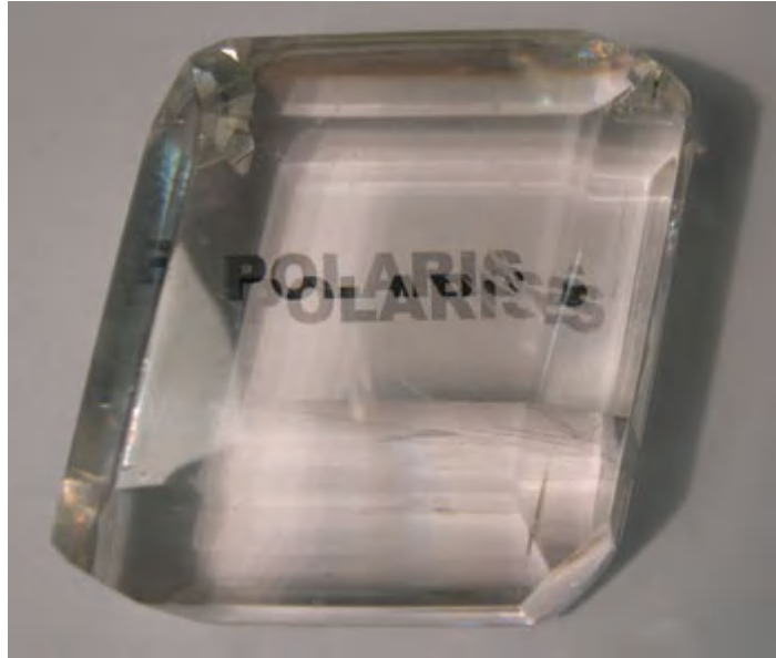
Figure 1.14 Light propagating through calcite divides into two modes, which follow different paths and generates two images.
