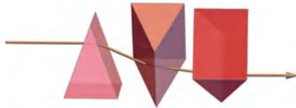
Figure 17.6 Three-prism example that refracts propagation vectors and forms a similar spherical polygon on the \mathbf{k} -sphere as the one shown in Figure 17.4.
