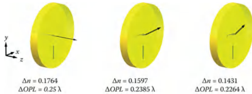
Figure 21.27 Three incident rays at 0.5\ \mu\text{m} along the principal section with incident angles 0^\circ , 30^\circ , and 45^\circ pass through a quarter wave A-plate and experience different birefringence \Delta n and \Delta OPL .
