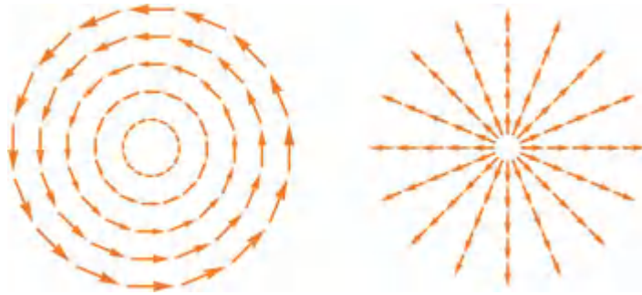
Figure 24.21 VAN-mode eigenpolarizations in a cell without pretilt, (left) ordinary mode is tangentially polarized, and (right) extraordinary mode is radially polarized. At normal incidence, the modes are degenerate; the ordinary and extraordinary modes have the same refractive index.
