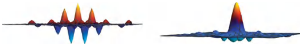
Figure 16.23 (Left) The (1, 1) component of the ARM is an interference pattern formed from the horizontal polarizer double slit JonesPupil(x, y) . The amplitude varies between -4.40 and 4.71 . (Right) The (2, 2) component of the ARM Fraunhofer diffraction pattern results from the vertical polarizer as a rectangular single slit JonesPupil(x, y) . The amplitude varies between -2.04 and 9.42 .
