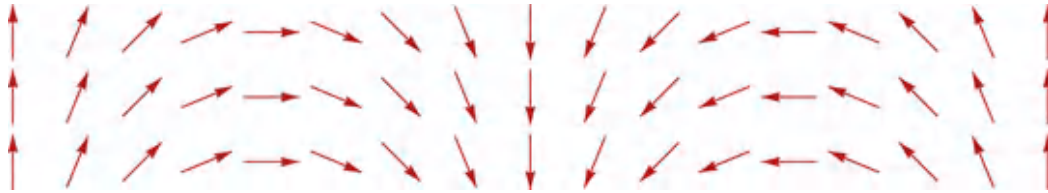
Figure 4.12 Addition of equal amplitude right and left circularly polarized beams with a 5% frequency difference yields a rotating linearly polarized state.
