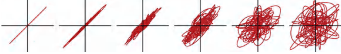
Figure 3.4 Examples of time-varying electric fields with randomly evolving polarization ellipses for partially linearly polarized light oriented at 45^\circ with DoLP of 1.0, 0.8, 0.6, 0.4, 0.2, and 0.
