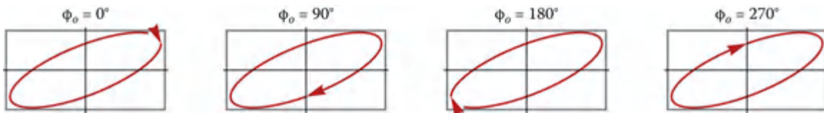
Figure 2.7 Polarization ellipses for E_x = 1 and E_y = e^{-i\pi/4}/2 for several phases \phi_o .
