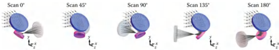
Figure 12.30 Ray trace figures showing a converging beam reflecting from fold mirror M1 (blue), then a scanning fold mirror M2 (magenta), and then incident on a detector (gray).
