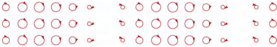
Figure 4.10 Insert a circular polarizer into the fringes of Figure 4.8 and the intensity fringes are recovered at a different phase.
