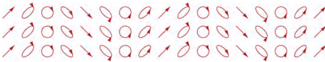
Figure 4.8 The interference of a horizontally polarized and vertically polarized beam of equal amplitude produces a periodic polarization state. The flux in these polarization fringes is constant. The maximum flux ( P_{\max} ) and the minimum flux ( P_{\min} ) are equal and the fringe visibility is zero.
