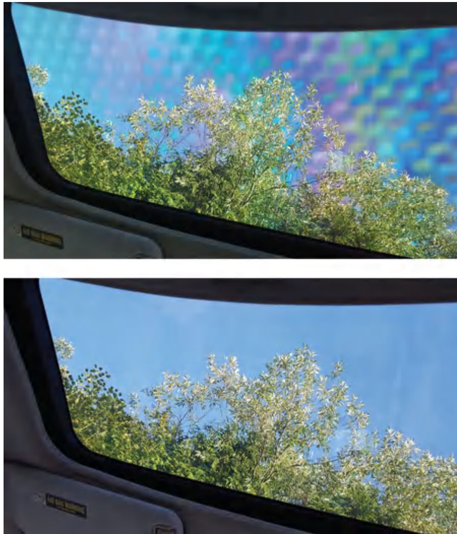
Figure 1.2 Moonroof photographed under a sunny day with (top) and without (bottom) a polarizer filter on the camera. The rainbow checkerboard pattern reveals the stress birefringence of the tempered glass.
