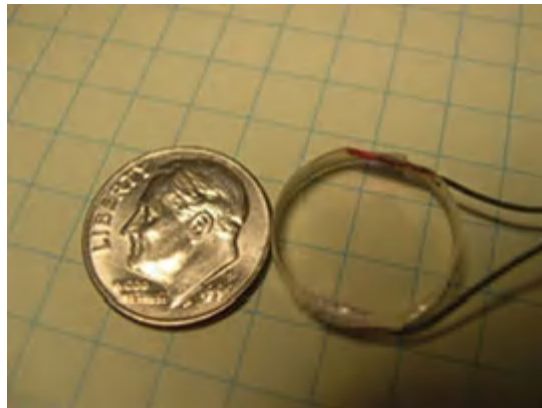
Figure 24.13 A small Fréedericksz cell retardance modulator for adjustable linear retardance. The LC is sealed between glass plates.
