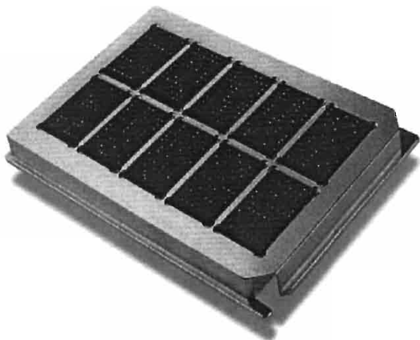
Fig. 5. Sample holder for 10 SpectroCHIPS for use in the SpectroSCAN mass spectrometer.
