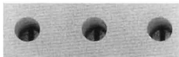
Fig. 3. A view of the cover plate displaying the holes created for the fluidics interconnection to the channels.
