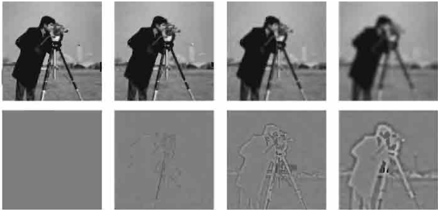
Fig. 2. Complex diffusion of the cameraman image for small theta ( \theta = \pi/30 ). Top - real values, bottom - imaginary values (factored by 20). Each frame (from left to right): original, image after times: 0.25, 2.5, 25.
