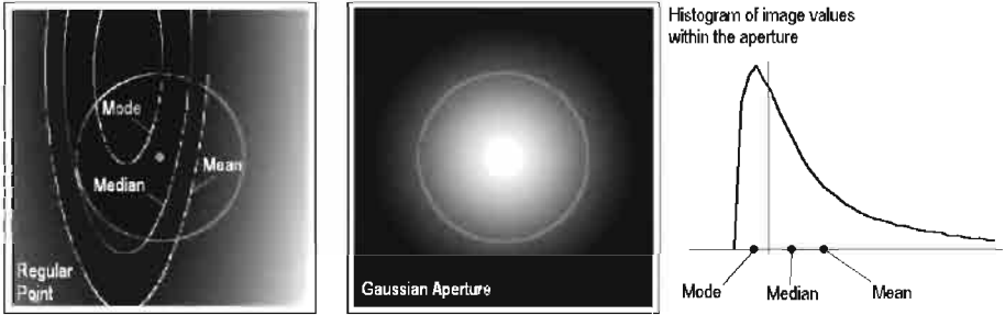
Fig. 1. The left panel shows an example image region centred on a regular point. The central panel shows a gaussian aperture. The right panel shows the histogram of the image at left within the aperture shown in the centre. The mean, median and mode of the histogram are marked, as are the corresponding isophotes in the underlying image on the left. The median isophote divides the image into two regions with equal integral of the aperture weighting.
