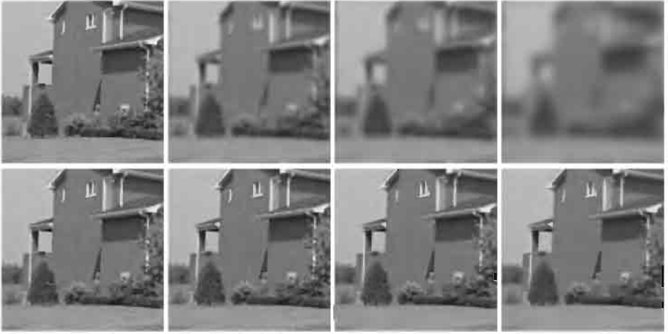
Fig. 2. Scale-space stack in RGB color-space. Top: Gaussian scale generator, from left to right: N = 0, 4, 7, 10 . Bottom: PMC diffusion with k = 4.5 . N = 0, 4, 7, 10 .
