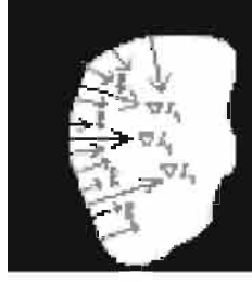
Fig. 3. An example of motion h = f - Id of a \xi -rigid deformation f for image I_1 . We show a level set of image I_1 , and the fields \nabla I_1 and h along its boundary. h varies only along the direction of \nabla I_1 .
