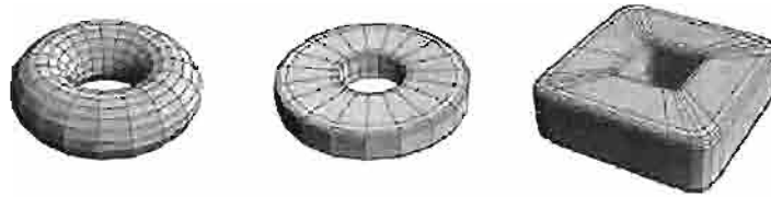
Figure 2. Examples of superquadric toroids. From left to right, we produce a round torus, a “pineapple-slice” toroid, and a square toroid. The north-south parameters, respectively, are 1.0, 0.2, 0.2, and the east-west parameters are 1.0, 1.0, and 0.2. The hole parameter, \alpha , is 2.
