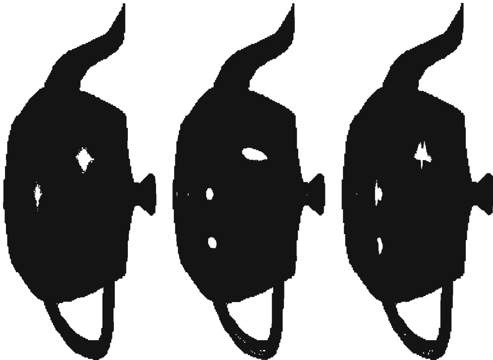
Figure 2. left: Gouraud shading, middle: Phong shading, right: Fence shading. Note: pictures have been rotated 90^\circ , so scanlines are now vertical.
