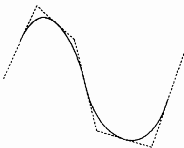
Fig. 6.3. Example of a B-spline curve ( M=3 )
