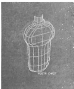
Fig. 6.29. Example of shape control on a surface of revolution (3)
