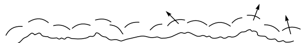
Fig. 12.8 Diffuse reflection of a plane wave front from a rough surface. It is evident that one does not have a well-defined reflected beam.
