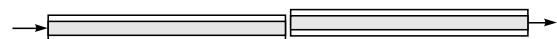
Fig. 29.4 A transverse alignment between two fibers would result in a loss of the optical beam.
