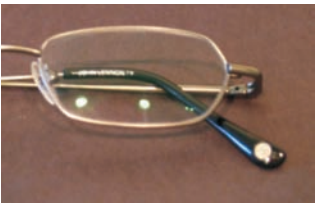
Chapter 15—Fig. 15.8 Comparison between an eyeglass lens without antireflective coating (top) and a lens with antireflective coating (bottom). Note the reflection of the photographer in the top lens and the tinted reflection in the bottom. The photograph was taken by Justin Lebar; used with permission from Mr. Lebar.
