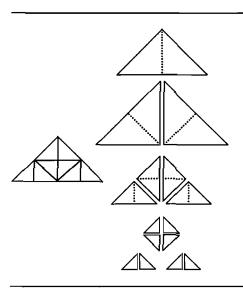
Figure 8.16 Subdivision of a triangle and the corresponding binary tree.
