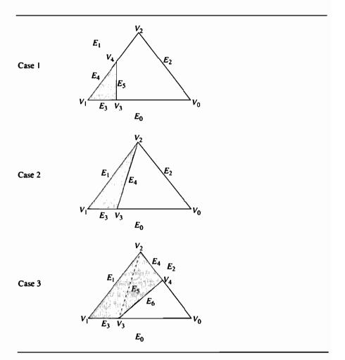
Figure 3.10 Three configurations for clipped triangle.
