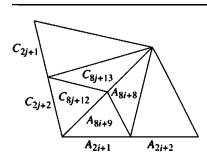
Figure 8.18 H-adjacency for triangles A and C.
