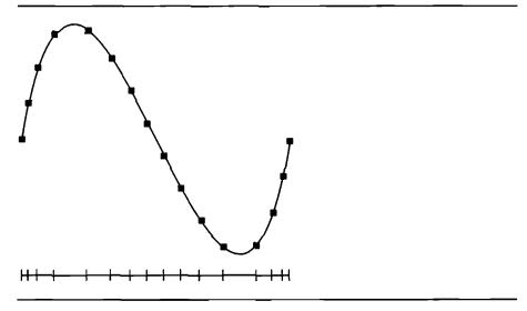
Figure 7.9 Subdivision of a curve by arc length.
