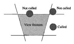
Figure 4.2 Examples of culled and unculled objects.
