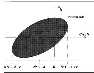
Figure 4.5 Projection of ellipsoid and frustum plane, no-cull case.
