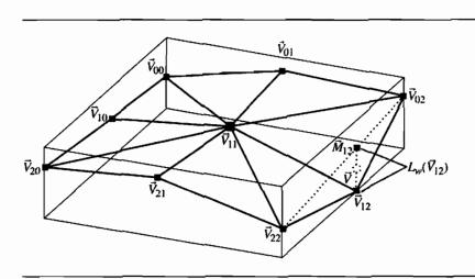
Figure 11.5 A single block with nine vertices labeled and all eight triangles drawn. The candidate vertex is  $\vec{V}_{12}$  and the candidate vertical line segment is  $\langle \vec{M}_{12}, \vec{V}_{12} \rangle$ . The midpoint of the segment is  $\vec{V}$  and the world height is  $L_w(\vec{V})$ . The corresponding screen space height is  $L_s(\vec{V})$ .
