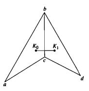
Figure 11.13 Adjacent triangles forming a nonconvex quadrilateral.
