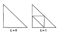
Figure 8.15 Subdivisions of parameter space for a triangle patch.
