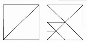
Figure 11.11 The left block is the configuration after block simplification. The right block is the configuration after vertex simplification.
