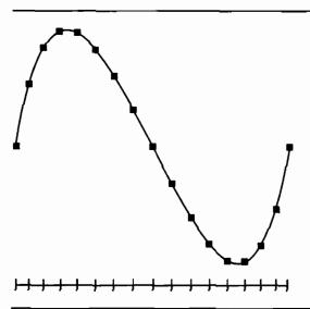
Figure 7.10 Subdivision of a curve by midpoint distance.
