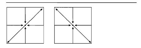
Figure 11.7 Vertex dependencies for an even block (left) and an odd block (right).
