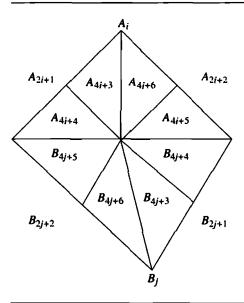
Figure 8.17 H-adjacency for triangles A and B.
