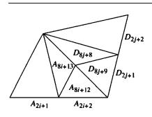
Figure 8.19 H-adjacency for triangles A and D.
