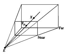
Figure 3.2 The standard camera model.
