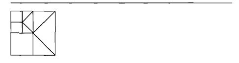
Figure 8.9 Partial subdivision illustrating the parent's topological constraint.
