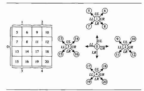
Figure 11.1 A  $5 \times 5$  height field and quadtree representation.
