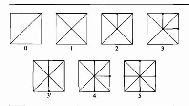
Figure 11.3 The seven distinct triangle configurations.
