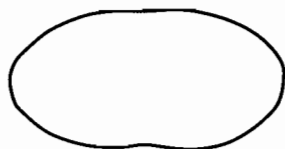
Figure 41 Mean of 10 randomly disturbed ellipses as in Fig. 39. This is an estimate of the ellipse contour function D(\varphi) .
